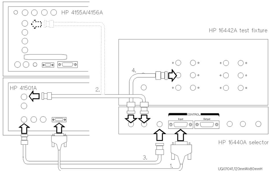
1. Connect the following by using a 3.0 m or 1.5 m control cable:
