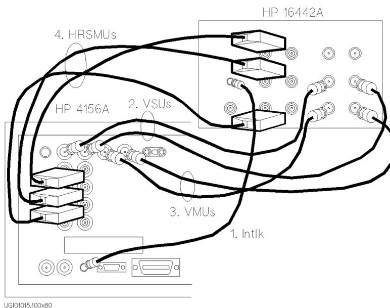
1. To prevent shock, *be sure* to connect following by 3.0m or 1.5m Intlk cable: Intlk terminal (HP 4156A)  $\leftrightarrow$  Intlk terminal (HP 16442A)
