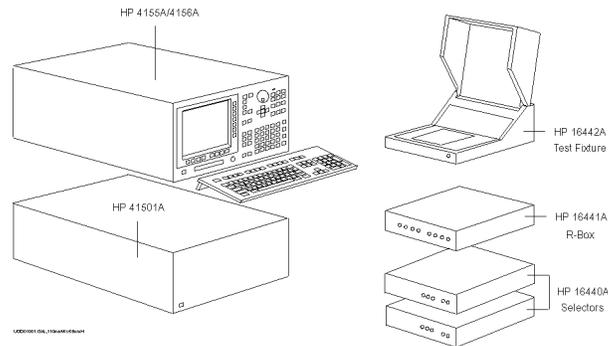
HP 4155A/4156A is a box type electronic measurement instrument with CRT display, flexible disk drive, operation keys, and interface connectors.
