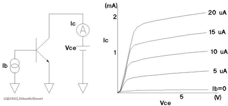
In the example above, a primary source ( $V_{ce}$ ) and a secondary source ( $I_b$ ) are defined. After primary sweep source finishes each sweep, the secondary sweep source outputs the next value.
