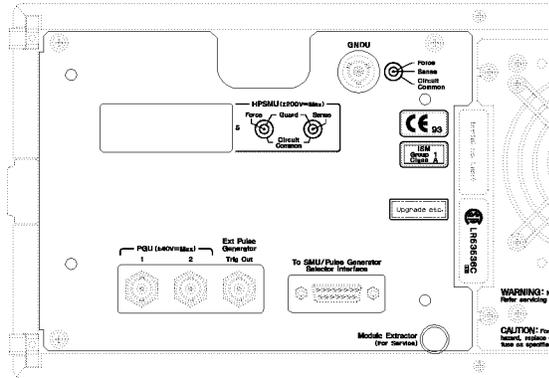
**Figure 1-4. Rear View of HP 41501A Option 402**
