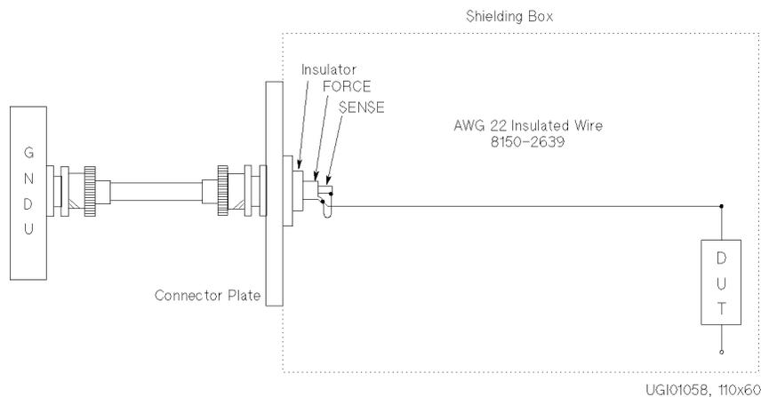
To easily connect GNDU for a measurement in which the accuracy is not important, connect only force to the DUT, without shorting sense and force.
