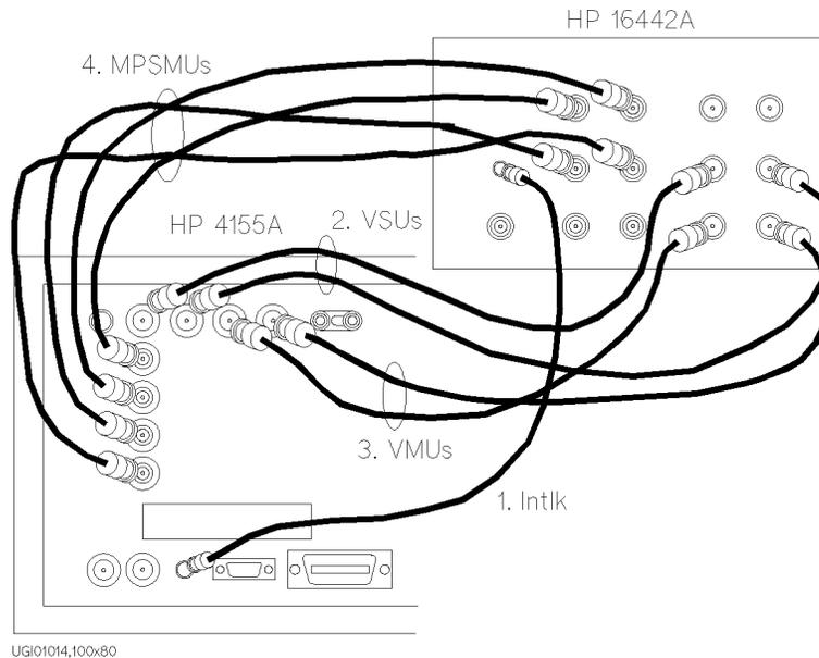
1. To prevent shock, *be sure* to connect following by 3.0m or 1.5m Intlk cable: Intlk terminal (HP 4155A)  $\iff$  Intlk terminal (HP 16442A)
