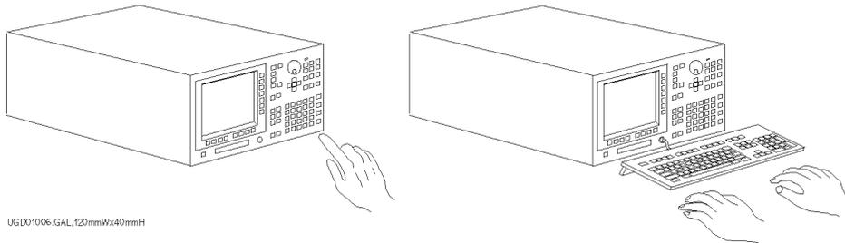
HP 4155A/4156A is operated by a “form fill-in” method. That is, the user-interface consists of setup and results pages, and you fill in fields on appropriate pages to select a measurement mode, set measurement parameters and conditions, set results display mode, and so on. After you execute the measurement, measurement results are displayed on result pages.
