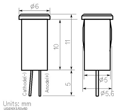
Figure 2-7. Dimensions of LED (HP part number 1450-0641)
