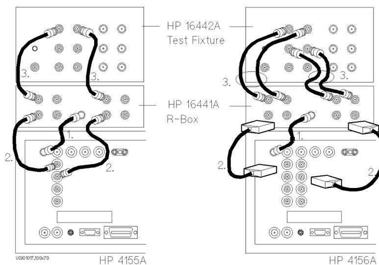
1. Connect the following by using a 3.0 m or 1.5 m control cable:
