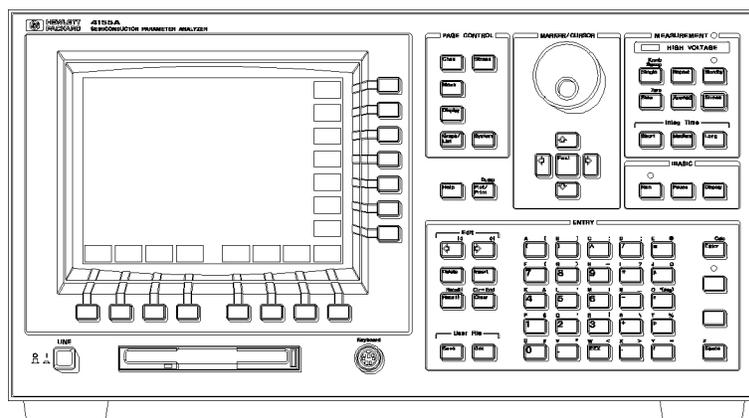
**Figure 1-1. Front View of HP 4155A/4156A**
