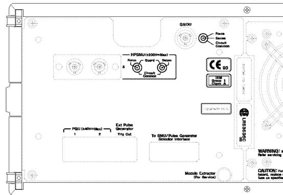
**Figure 1-5. Rear View of HP 41501A Option 410**
