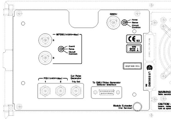
**Figure 1-8. Rear View of HP 41501A Option 422**
