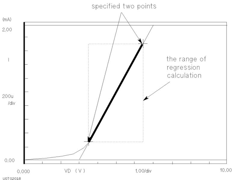
Data condition mode specifies a point related to the measurement curve. So, if no measurement data satisfy the specified condition, the nearest measurement point is used.
