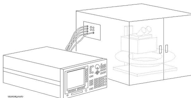
1. Before installing connector plate, make sure that HP 4155A/4156A and HP 41501A are turned off.
