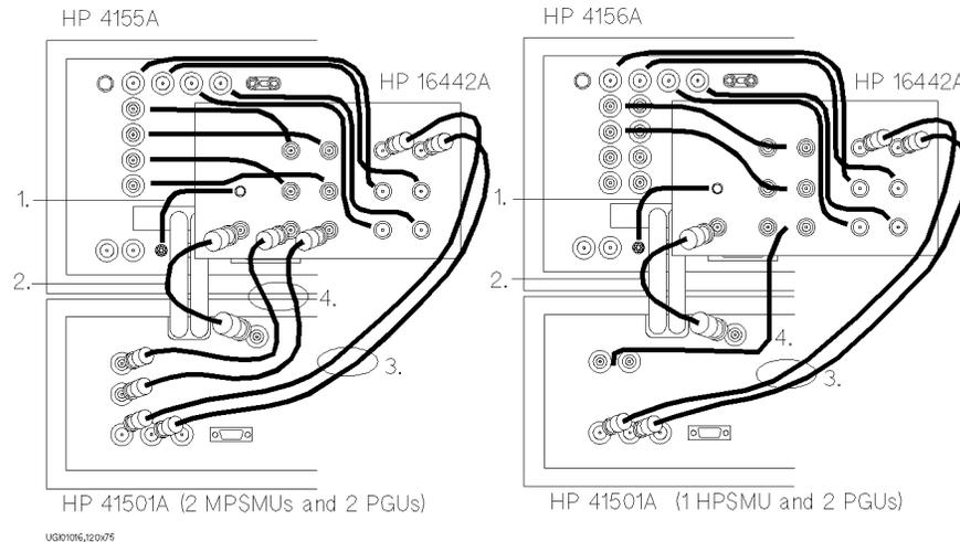
1. To prevent electric shock, make sure that Intlk terminal of HP 4155A/4156A is connected to Intlk terminal of HP 16442A.
