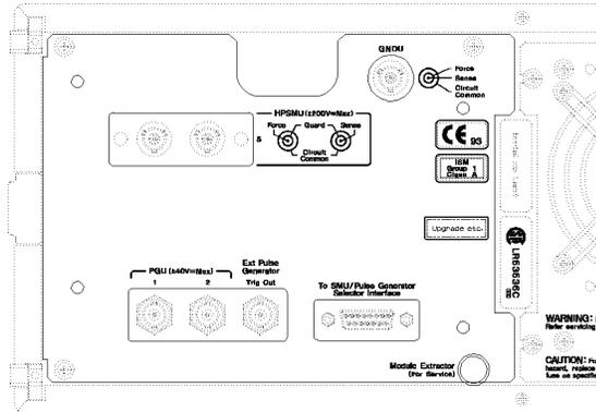
**Figure 1-6. Rear View of HP 41501A Option 412**
