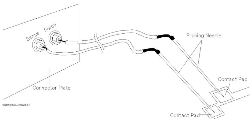
To reduce the leakage current, use coaxial cables to connect the connector plate to the probing needle.
