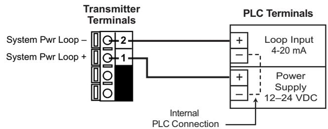
Example: Two transmitters connected to PLC/Recorder with separate power supply
