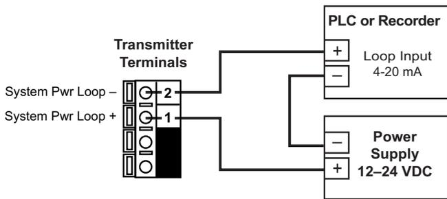
Connection to a PLC with built-in power supply
