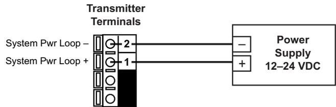
Connection to a PLC/Recorder, separate supply
