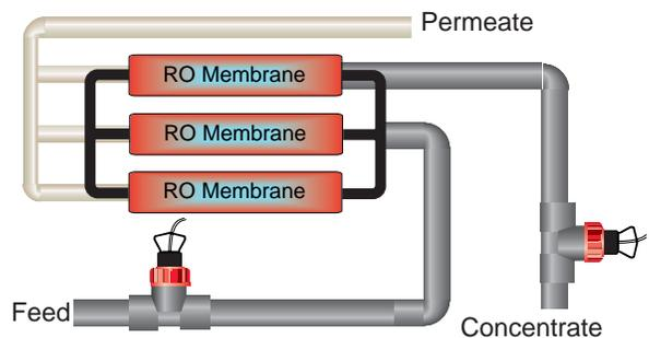
**% Recovery C:**  $[(\text{Feed} - \text{Concentrate}) \div \text{Feed}] \times 100$
