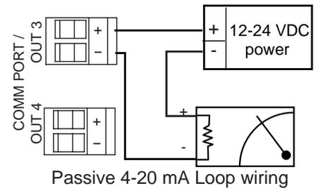
Passive 4-20 mA Loop wiring
