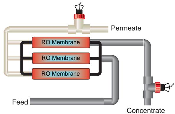
**% Recovery B:**  $\text{Permeate} \div (\text{Permeate} + \text{Concentrate}) \times 100$
