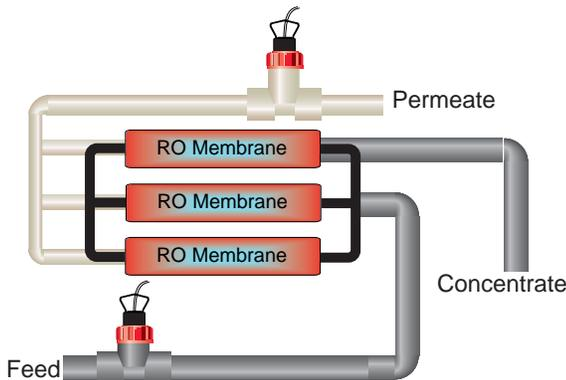
**% Recovery A:**  $(\text{Permeate} \div \text{Feed}) \times 100$
