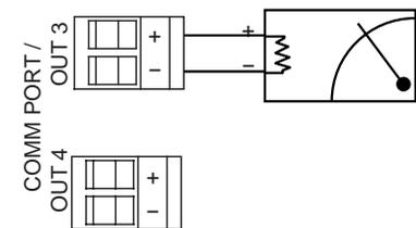
0-5 VDC Output wiring
