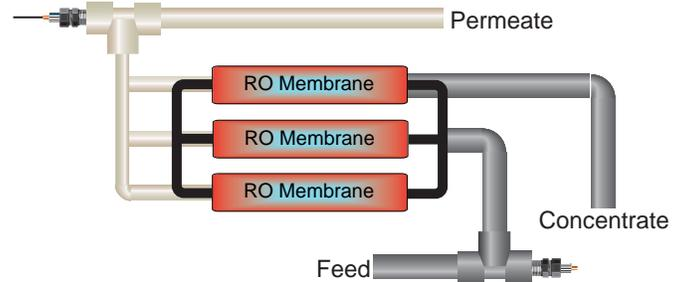
**% Passage:**  $(\text{Permeate} \div \text{Feed}) \times 100$
