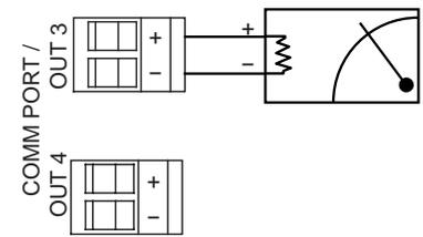
Active 4-20 mA Loop wiring
