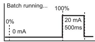
• **Current Output - End of Batch (sec. 8C):** This function is designed to trigger a second 5600 batch controller's remote START input for a second batching stage. When the batch starts, the current output remains at 0 mA until the end of the batch, then jumps to 20 mA for 500 milliseconds. The 500 millisecond current pulse triggers the second 5600's remote START terminal to start the second batch stage.
