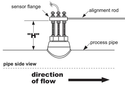
After correct dimensions are calculated and recorded, the sensor can be installed in the fitting. The Standard and Hot-Tap versions require substantially different procedures.
