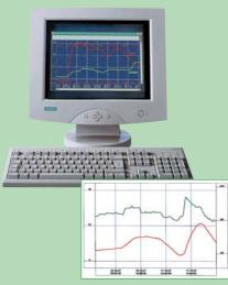
Comfortable data evaluation (with graphic or table layout) of the saved data via RS 232 interface in connection with PC software (included in delivery).
