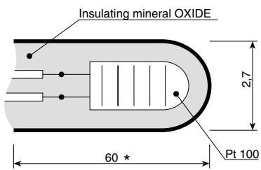
\* Minimum length of immersion to perform measurement correctly
