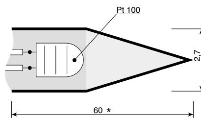
\* Minimum length of penetration to perform measurement correctly
