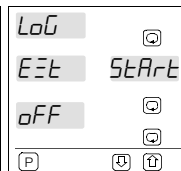
Data logger Start/Stop when trigger source ≠ OFF
