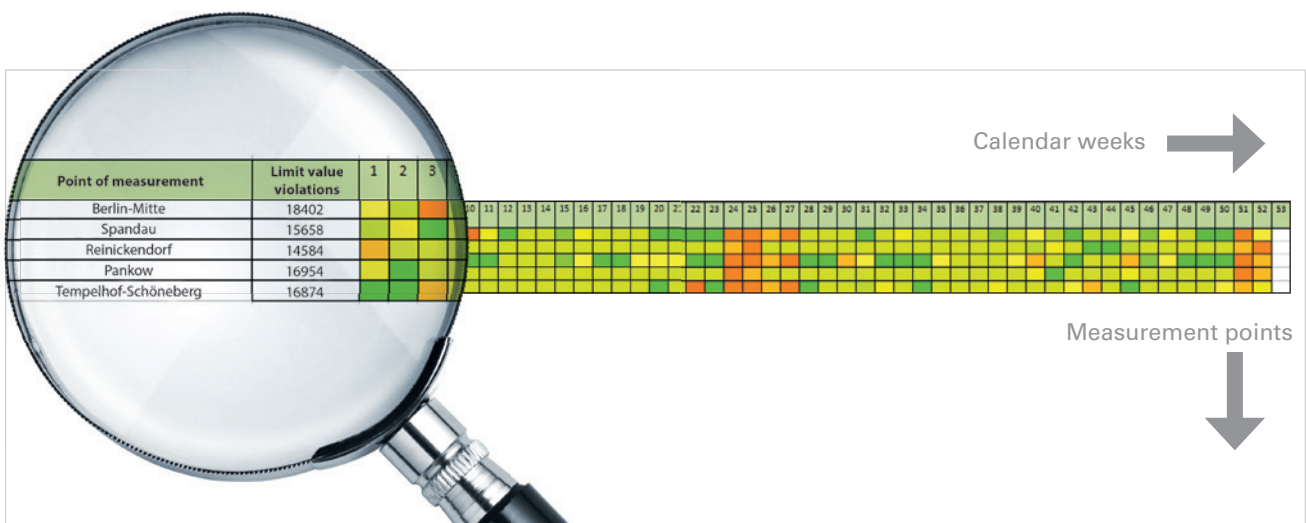
Fig.: Heatmap, i.e. colour (traffic light principle) illustration of how good or bad the power quality was at a particular measurement point in a calendar week. 图:热图,即颜色(交通灯原理),说明在一个日历周的特定测量点的电能质量是好是坏。这一原则保证了对整个供应区域的快速概览。
