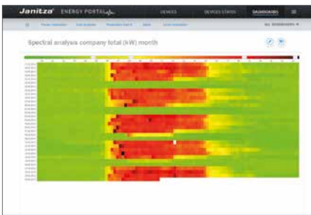
Heat map (spectral analysis) to determine peak loads that drive costs. The scroll bar in the chart's header area can be used to adjust the threshold values individually.
