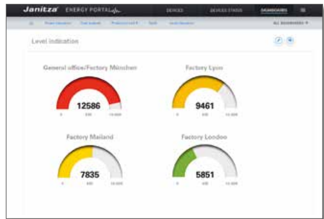
Benchmark for the production sites with level displays. The limit values can be adjusted individually for each of the locations.
