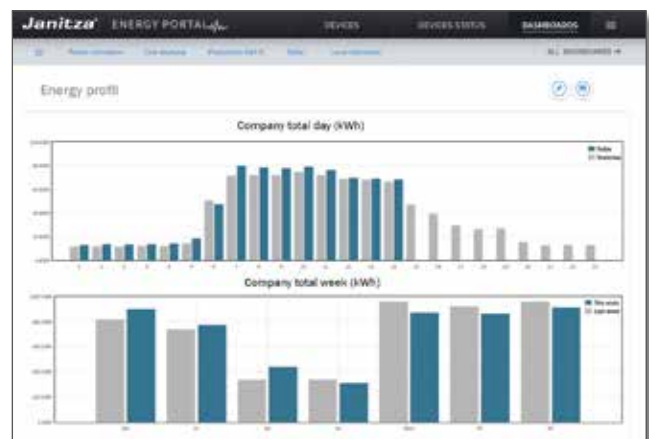
Dashboard example with two bar charts to compare el. energy values from the current day with the previous day or the current week with the previous week.
