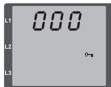
Fig. Password prompt If a password was set, it can be entered with buttons 1 and 2.
