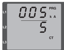
Fig. Current transformer programming mode Buttons 1 and 2 can be used to modify the primary and secondary current (cf. page 51).
