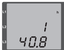
Fig. Measured value screen Operating hours counter The UMG 96RM-PN shows the number 140.8 hrs in the operating hours counter. This corresponds to 140 hours and 80 industry minutes. 100 industry minutes correspond to 60 minutes. In this example, the 80 industry minutes correspond to 48 minutes.
