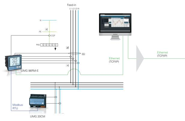
Fig.: The 20 channels of the UMG 20CM can be optionally used for residual current or operational current monitoring by utilising the corresponding current measurement transformer. In the case of residual current monitoring, the residual currents flowing to ground or any other path are acquired.
