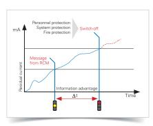
Fig.: Message before shut-down - an objective of residual current monitoring
