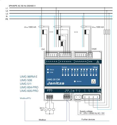
Recommendation: The bus should not contain more than 10 devices, type UMG 20CM if several UMG 20CM measuring channels are used. If the APP "20CM-Webmonitor" is used, the number is limited to 5 devices due to the APP management).
