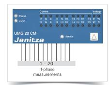
Fig.: 20 single-phase operating current or RCM measurements
