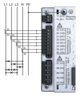
Fig. "Current measurement via current transformers" connection example.
