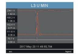
Fig. Illustration of the half wave effective values for an event
