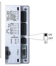
Fig. Termination via DIP switch activated (ON).
