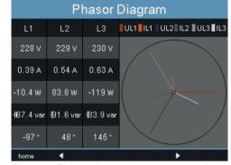
Fig. In the Phasor diagram, the voltages are displayed with long phasors and the currents with short phasors.
