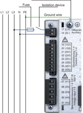
Fig. Example connection for the supply voltage
