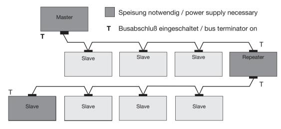
Fig. Bus structure illustration
