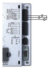
Fig. Connection of digital outputs
