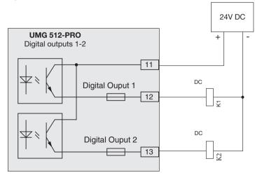
Fig. Example for connecting 2 relays to digital outputs 1 and 2
