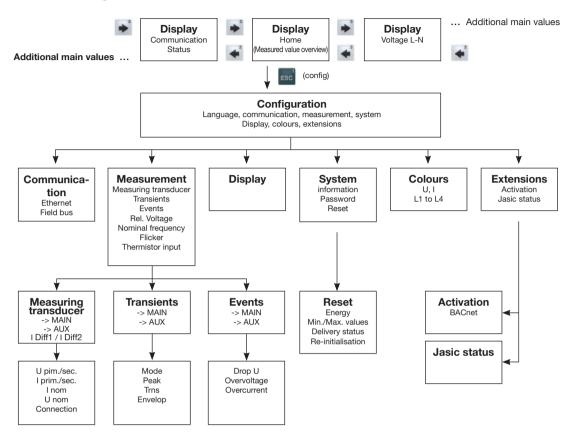
Fig. Schematic illustration of the menu guide for the configuration menu
