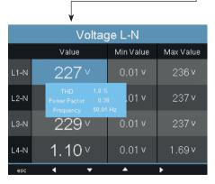
Fig. Additional information for L1-N voltage
