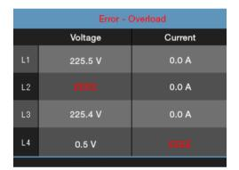
Fig. Indication of values exceeding the measurement range in voltage circuit L2 and in current path I4
