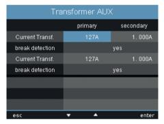
Fig. Residual current transformer menu
