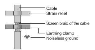
Fig. Shielding procedure at cabinet entry.
