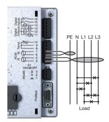
Fig. "Residual current monitoring via current transformers" connection variant
