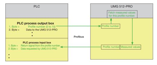
Fig. Block diagram for data exchange between PLC and UMG 512-PRO.
