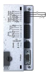
Fig. Connection of digital inputs
