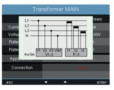
Fig. Example for measurement in a threephase 4-conductor network with asymmetric loading
