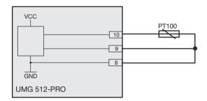
Fig. Connection example for temperature measurement with a PT100
