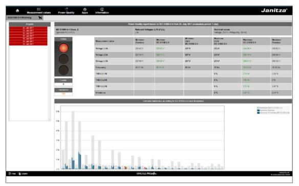
Fig. IEC 61000-2-4 parameters with traffic-light principle
