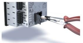
Fig. Replacing the battery using long-nose pliers
