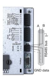
Fig. RS485 connection example
