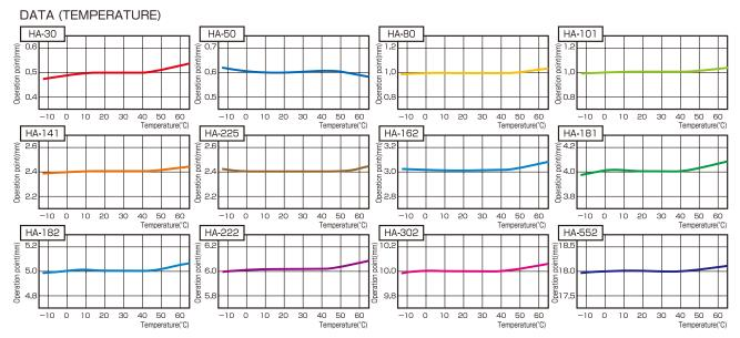
Condition of measuring :Operating distance is set by 50% of stable operating distance, fixed condition of measuring object (Feø90), the temperature shall be changed by  $\pm 10^{\circ}$ C per hour from the basing temperature of 23°C, data is collected when the temperature is stable.
