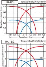
object which is horizontally moved at detection face.
