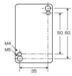
DIN rail mountable (Conform to DIN46277)
