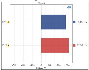
The Multitone Analyzer: DC Level result uses the multitone method to measure dc level in the presence of signal for each DUT channel, displayed as a meter (single value) result. If AC Coupled is selected in the analog input configuration settings in Signal Path Setup, the Multitone Analyzer: DC Level result is not available. Change the setting to DC Coupled and start the measurement again.
