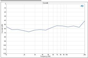
This result shows the crosstalk introduced into Channel 1 from Channel 2, with both channels driven but the Channel 1 connection between the generator and the DUT disconnected.
