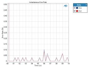
The Digital Error Rate: Instantaneous Error Rate measurement result provides a record of the rate of digital errors versus elapsed time.
