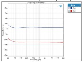
Group delay is a measure of the rate of change of phase shift as a function of frequency. Group delay can also be described as a time delay of a group of frequencies with respect to the generator.
