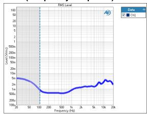
The Level result provides a graphical display of the frequency response of the loudspeaker.
