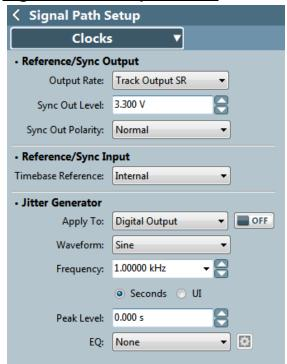
The features and controls described here require the Advanced Master Clock, a standard feature on the APx555 and an option on modular APx analyzers. When the Advanced Master Clock is present, these inputs and outputs are available on connectors on the APx rear panel.
