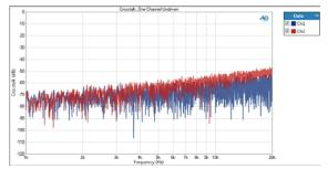
The Crosstalk, One Channel Undriven result is a continuous sweep measurement that provides a graphi-
