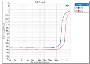
The Stepped Level Sweep: THD+N Level result uses a sine wave stimulus signal that is moved across a range of levels in a series of points. X axis is generator level; Y axis is DUT output THD+N level.
