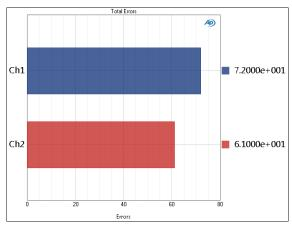
The Digital Error Rate: Total Errors measurement result provides a single-value measurement of the total digital errors acquired.
