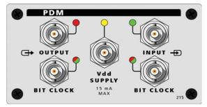
The PDM option provides a complete solution for addressing circuits or devices with a PDM input or out-
