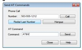
You can open the Send AT Commands dialog by clicking Actions > AT Commands from Signal Path Setup, or from the context menu opened by right-clicking in the Bluetooth Monitor.
