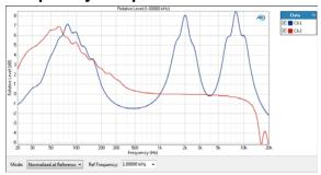
The Frequency Response: Relative Level result is a continuous sweep measurement that provides a graphical display of the frequency response of each channel. In this result the DUT output level is plotted against frequency, relative to the level at a selected frequency. This enables you to specify the frequency that will be set as 0 dB and view the response in relation to that frequency. A midband frequency such as 1 kHz is often set as the reference frequency, and is the default here.
