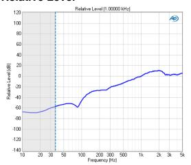
The Relative Level result is a continuous sweep measurement that provides a graphical display of the frequency response of the loudspeaker. In this result the DUT output level is plotted against frequency, relative to the level at a selected frequency set in the **Ref Frequency** field.
