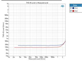
The Stepped Level Sweep: THD+N Level vs. Measured Level result uses a sine wave stimulus signal that is moved across a range of levels in a series of points. X axis is measured DUT output level; Y axis is DUT output THD+N level.
