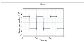
1 kHz digital square wave, 192 kHz SR
