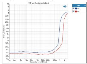
The Stepped Level Sweep: THD Level result uses a sine wave stimulus signal that is moved across a range of levels in a series of points. X axis is generator level; Y axis is DUT output THD level.
