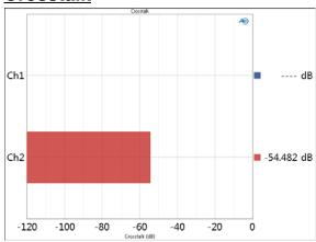
The Crosstalk measurement result provides a singlevalue measurement crosstalk in the DUT. In this case, the Channel 2 drive signal has been interrupted in the DUT, so crosstalk results only appear in Channel 2.
