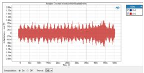
The Acquired Crosstalk Waveform, One Channel Driven result is a continuous sweep measurement that displays the Acquired Crosstalk Waveform for each undriven channel. This acquisition is only made when Crosstalk Mode is set to **High Accuracy, One Channel Driven**. See page 220 for more information about acquired waveform.
