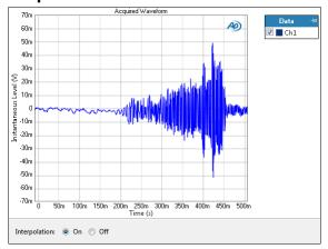
The Acquired Waveform view is a continuous sweep measurement that displays the acquired waveform for each channel. Acquired waveform is plotted against time.
