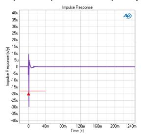
This is a Loudspeaker Production Test Impulse Response result from a system that has reversed polarity. The primary impulse is negative. Notice that the limit set at –18u has been crossed and a limit failure marker has been set.
