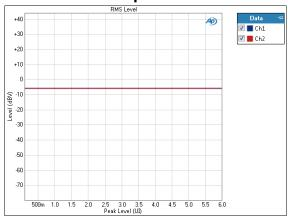
The **Jitter Level Sweep: RMS Level** result uses a fixed audio stimulus signal while the jitter generator is moved across a range of levels in a specified number of points. X axis is generator level; Y axis is DUT output level.
