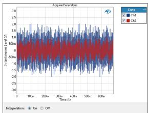
The **Multitone Analyzer: Acquired Waveform** result provides a time domain display of the acquired signal.
