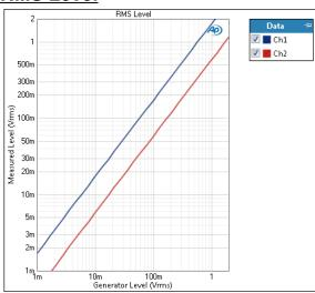
The Bandpass Level Sweep: RMS Level result uses a sine wave stimulus signal that is moved across a range of levels in a series of points. X axis is generator level; Y axis is the bandpass filtered DUT output level
