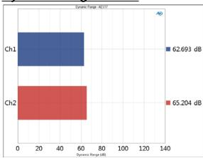
The Dynamic Range (AES17) measurement provides a single-value result showing the AES17 Dynamic Range for each DUT channel.
