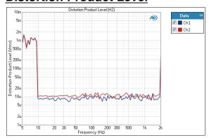
The Jitter Frequency Sweep Distortion Product Level result uses a fixed audio stimulus signal while the jitter generator is moved across a range of frequencies in a specified number of points. In this result the level of the selected harmonic distortion product in the DUT output is plotted against frequency.
