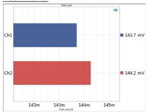
Peak Level provides a single-value meter result, displaying of the peak output level from each DUT channel, as measured at each analyzer input.
