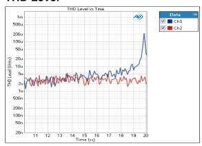
The Measurement Recorder: THD Level measurement result provides a record of THD level versus elapsed time for any audio signal. The illustration shows a 20-second record of a 10 kHz sine wave on two channels, with a 10 kHz EQ control adjusted from about -20 dB to about +12 dB during the course of the recording.
