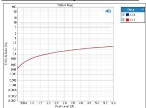
The Jitter Level Sweep: THD+N Ratio result uses a fixed audio stimulus signal while the jitter generator is moved across a range of levels in a specified number
