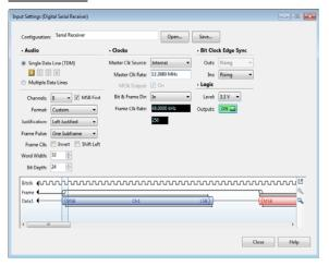
This dialog allows you to set, save or load digital serial receiver configurations. A dynamic timing diagram provides an on-screen display of your configuration settings. Receiver connections are provided on an HD-15 connector, with Master Clock, Frame Clock, Bit Clock, Channel Clock and four Data line connections. A monitor connector provides buffered outputs of these signals for oscilloscope monitoring.
