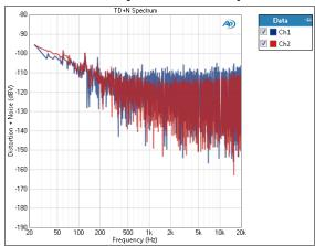
The Multitone Analyzer: TD+N Spectrum result provides an FFT spectrum display of the acquired signal. All bins, odd and even, that are not tone bins nor within the current **Skirt width** are plotted in this display. This removes the stimulus tones and reports a total distortion + noise result.
