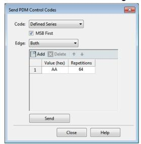
The PDM transmitter can embed amplifier control codes in the PDM bitstream. Click the **Send Codes: Settings** button in the PDM Monitor panel to open the Send PDM Control Codes dialog.
