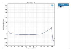
The THD+N Level result plots the DUT measured THD+N output level on the Y axis, against the generator frequency on the X axis. This method is often employed to plot an amplifier frequency sweep at the amplifier's maximum output level.
