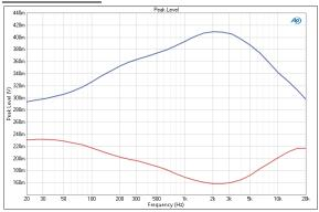
Bandpass Frequency Sweep: Peak Level results uses a sine wave stimulus signal that is moved across a range of frequencies in a specified number of points. This is a frequency response sweep, bandpass filtered, with peak-scaled results.
