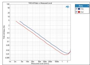
The Stepped Level Sweep: THD+N Ratio vs. Measured Level result uses a sine wave stimulus signal that is moved across a range of levels in a series of points. X
