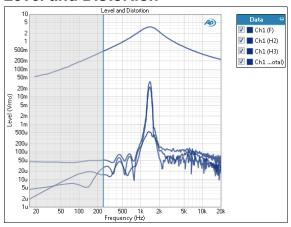
The Acoustic Response: Level and Distortion result is a continuous sweep measurement that provides a graphical display of the fundamental level vs. frequency and the distortion level vs. frequency of the loudspeaker connected to each channel, plotted on the same graph. Distortion curves included total distortion level, H2 distortion level and H3 distortion level.
