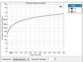
The Jitter Level Sweep Distortion Product Level result uses a fixed audio stimulus signal while the jitter generator is moved across a range of levels in a specified number of points. In this result the level of the selected harmonic distortion product in the DUT output is plotted against generator level.
