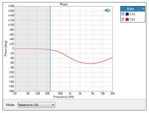
The Acoustic Response Phase result is a continuous sweep measurement that displays the DUT output phase for each channel, plotted against frequency.
