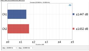
The Bandpass Frequency Sweep: Deviation result uses a sine wave stimulus signal that is moved across a range of frequencies in a specified number of points. This result is a single value measurement computed from the stepped sweep that shows the frequency deviation (the total range of frequency variation) of each channel as a meter bar. You can specify a minimum and maximum frequency to define the range of the deviation measurement.
