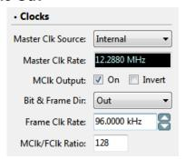
Receiver Settings: Master Clk Internal, Bit & Frame Out
