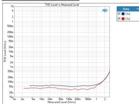
The Stepped Level Sweep: THD Level vs. Measured Level result uses a sine wave stimulus signal that is moved across a range of levels in a series of points. X axis is measured DUT output level; Y axis is DUT output THD level.
