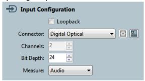
Digital Optical enables the digital optical input, available on a Toslink connector on the instrument front panel.
