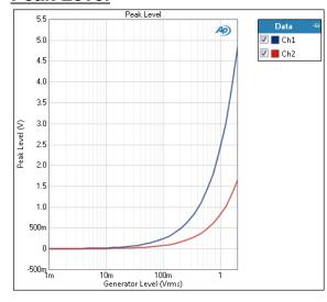
The Bandpass Level Sweep: Peak Level result uses a sine wave stimulus signal that is moved across a range of levels in a series of points. X axis is generator level; Y axis is the bandpass filtered DUT output level, scaled in peak units.
