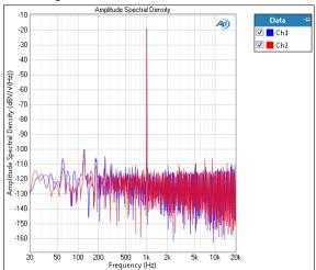
The Signal Analyzer is a general purpose diagnostic tool that uses a high-resolution FFT technique to provide several different display results. Amplitude Spectral Density is a frequency domain result, displaying the signal amplitude per root Hertz, versus frequency.
