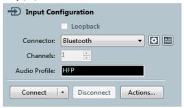
Note: The Bluetooth choice is only available for analyzers fitted with the APx Bluetooth Option module.
