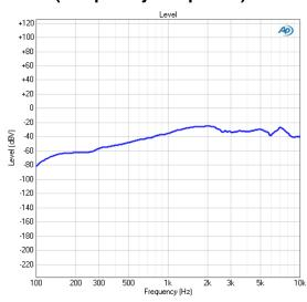
Loudspeaker Production Test: Level is a continuous sweep result that displays level plotted against frequency. This is the frequency response of the loudspeaker.
