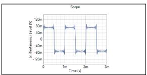
1 kHz digital square wave, 48 kHz SR
