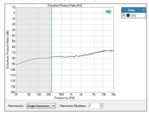
The Acoustic Response Distortion Product Ratio result is a continuous sweep measurement that provides a graphical display of the selected harmonic distortion products present in each channel. In this result the ratio of the level of the selected harmonic distortion product to the fundamental in the DUT output is plotted against frequency.
