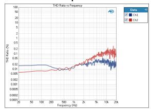
The THD Ratio result is a continuous sweep measurement that provides a graphical display of the harmonic distortion response of each channel. In this result the ratio of the level of the THD (total harmonic distortion) to the fundamental in the DUT output is plotted against frequency.
