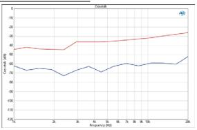
This result shows the crosstalk introduced into Channel 1 from Channel 2, and the crosstalk introduced into Channel 2 from Channel 1.
