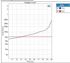
The Bandpass Level measurement result provides a record of the Bandpass Level versus elapsed time for any audio signal. The illustration shows a 20-second record of a 10 kHz sine wave on two channels, with a 10 kHz EQ control adjusted from about -20 dB to about +12 dB during the course of the recording.
