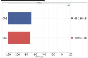
The DIM Ratio result provides single-value measurement results of the IMD (intermodulation distortion) ratio in the output signal from each DUT channel.
