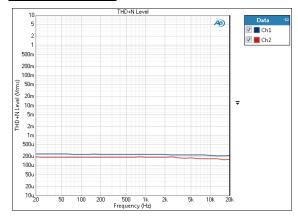
The THD+N Level result is a stepped frequency sweep measurement that provides a graphical display of the THD+N response of each channel. In this result the level of the THD+N (total harmonic distortion plus noise) in the DUT output is plotted against frequency.
