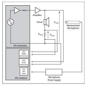
This configuration is enabled when **Test Configuration** is set to **External (2 Ch)** and the analyzer inputs are set to unbalanced.
