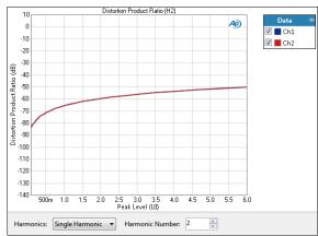
The Jitter Level Sweep Distortion Product Ratio result uses a fixed audio stimulus signal while the jitter generator is moved across a range of levels in a specified number of points. In this result the ratio of the level of the selected harmonic distortion product to the fundamental in the DUT output is plotted against generator level.
