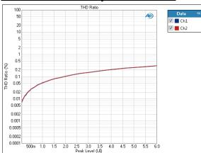
The Jitter Level Sweep: THD Ratio result uses a fixed audio stimulus signal while the jitter generator is moved across a range of levels in a specified number of points. X axis is generator level; Y axis is DUT output THD ratio.
