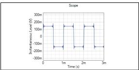
1 kHz digital square wave, 96 kHz SR
