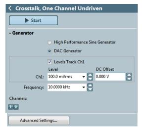
To run Crosstalk, One Channel Undriven, click **Start**. The generator will output the test signal to the DUT on all channels except Channel 1. After the first result is displayed, the measurement runs again with Channel 1 turned **ON**, and Channel 2 **OFF**. This process repeats through all of the available channels. Read the crosstalk measured in each remaining channel from the meter bar display.
