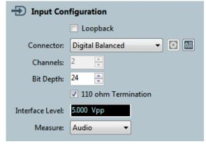
Digital Balanced enables the balanced digital electrical input, available on an XLR female connector on the instrument front panel. This input is optimized to accept signal at the professional signal level for balanced signals compatible with AES3 and IEC60958-4 (5 Vpp).
