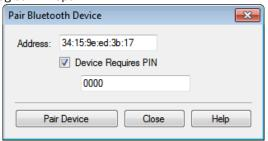
Some devices may require the exchange of a PIN code. The APx Bluetooth PIN code is set to 0000; a field in the pairing dialog allows input of a remote device's PIN code.
