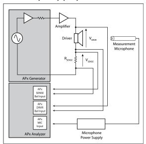
This is our recommended configuration when making a 2-channel impedance measurement. This configuration is enabled when **Test Configuration** is set to **External (2 Ch)** and the analyzer inputs are set to balanced.
