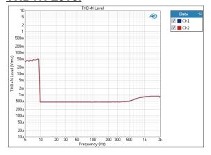
The THD+N Level result uses a fixed audio stimulus signal while the jitter generator is moved across a range of frequencies in a specified number of points. In this result the level of the THD+N (total harmonic distortion plus noise) in the DUT output is plotted against frequency.
