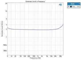
The Level result plots the generator output level on the Y axis, against the generator frequency on the X axis.
