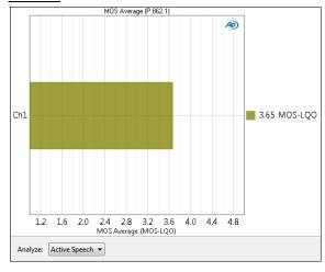
The PESQ: MOS Average result is the primary result for the PESQ (Averaged) measurement. The PESQ score is mapped to MOS-LQO using P.862.1 for narrowband analysis, or P.862.2 for wideband analysis. This result
