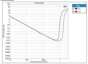
The Stepped Level Sweep: THD+N Ratio result uses a sine wave stimulus signal that is moved across a range of levels in a series of points. X axis is generator level; Y axis is DUT output THD+N ratio.
