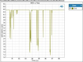
The PESQ: MOS vs Time is useful for cause analysis. The result shows a graph of the MOS score versus elapsed time.
