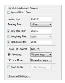
Typical Analyzer controls (Measurement Recorder shown)
