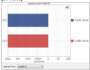
The Multitone Analyzer: Maximum Level (at Tone) result uses the multitone method to provide the calculated maximum level for a selected tone for each DUT channel, displayed as a meter (single value) result.
