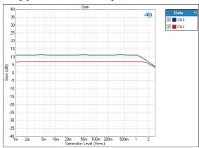
The Stepped Level Sweep: Gain result uses a sine wave stimulus signal that is moved across a range of levels in a series of points. X axis is generator level; Y axis is gain in the DUT. Gain is a ratio, calculated by dividing the DUT output level by the generator level.
