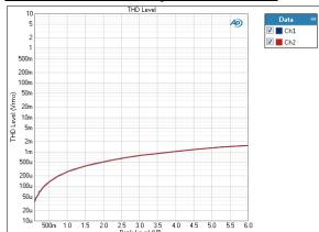
The Jitter Level Sweep: THD Level result uses a fixed audio stimulus signal while the jitter generator is moved across a range of levels in a specified number of points. X axis is generator level; Y axis is DUT output THD level.
