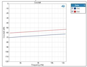
The **Multitone Analyzer: Crosstalk** result uses the multitone method to provide a graphical display of the crosstalk vs. frequency (crosstalk response) for each channel of the DUT. The crosstalk of each tone pair is measured, and a response curve is plotted through these values.
