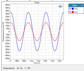
The Signal Analyzer is a general purpose diagnostic tool that uses a high-resolution FFT technique to provide several different display results. Scope is a time domain result, displaying the signal amplitude versus time, analogous to an oscilloscope view.
