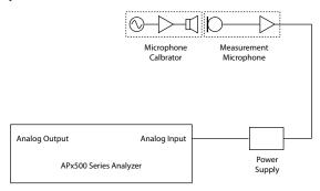
Two calibration levels are in standard use for acoustic calibration: 94 dB SPL and 114 dB SPL. If both are available on your calibrator, select the level most suited to your measurement. Mount the calibrator firmly on the microphone capsule and turn it ON.
