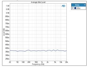
**Stepped Frequency Sweep: Average Jitter Level** results uses a sine wave stimulus signal that is moved across a range of frequencies in a specified number of points.
