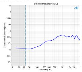
The Loudspeaker Production Test Distortion Product Level result is a continuous sweep measurement that provides a graphical display of the selected harmonic distortion products. In this result the level of the selected harmonic distortion product in the DUT output is plotted against frequency.
