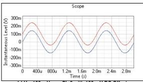
1 kHz, 100 mVrms; Ch 2 with 100 mV DC Offset.
