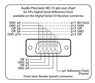
The clock signal appears on pin 5 of the Digital Serial I/O Receiver HD15 jack. Pins 2, 4, 6, 7, 10, 12 and 14
