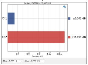
Continuous Sweep Deviation is a single value result computed from the continuous sweep acquisition. In this result the frequency deviation (the total range of frequency variation) of each channel is displayed as a meter bar. You can specify a minimum and maximum frequency to define the range be considered in the deviation measurement.
