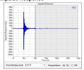
The Impulse Response provides a graphical display of the IR of the loudspeaker and acoustic space. This view is useful in setting up an acoustic measurement in conjunction with the Energy Time Curve view, using the Time Window. For more information about impulse response, see page 218.
