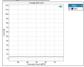
The Bandpass Level Sweep: Average Jitter Level result uses a sine wave stimulus signal that is moved across a range of levels in a series of points. X axis is generator level; Y axis is the bandpass filtered DUT output jitter level, scaled in average units.
