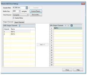
The ASIO Settings dialog provides a panel to set buffer size and clock source, and to map the ASIO device output and input channels to the APx analyzer output and input channels. From this dialog, you can also open the device control panel (when supported), and view device information (when supported).
