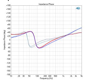
This result provides a graphical display of the impedance phase response of the driver, plotting the impedance phase versus frequency. The dashed line is the model fit trace, here using the Standard model. Traces for **Added Mass** are also shown.
