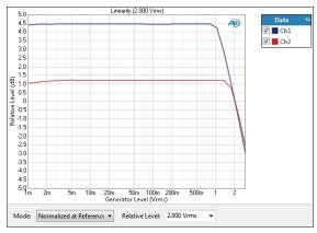
The Stepped Level Sweep: Linearity result uses a sine wave stimulus signal that is moved across a range of levels in a series of points. X axis is generator level; Y axis is linearity in the DUT. Linearity is a ratio, calcu-
