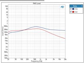
Stepped Frequency Sweep: RMS Level results uses a sine wave stimulus signal that is moved across a range of frequencies in a specified number of points. This is the conventional frequency response sweep.
