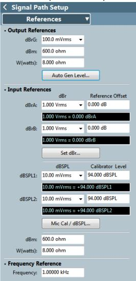
A signal path through a DUT will have an optimal operating level for each measurement. This level may be specified in a device's specifications, required for a standard measurement method, or may be determined on the bench by a monitoring a parameter such as distortion.
