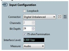
This selection enables the unbalanced digital electrical input, available on a BNC connector on the instrument front panel.
