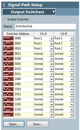
Audio Precision manufactures optional switchers that can be used to connect or disconnect many signal channels (up to 192 input and 192 output channels) to or from the instrument, under software control. See general switcher operating information beginning with the Switchers topic.
