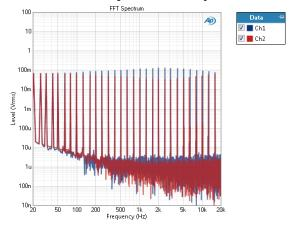
The **Multitone Analyzer: FFT Spectrum** result provides an FFT spectrum display (a frequency domain display) of the acquired signal. Every bin is plotted in this display. For a multitone stimulus, this will show the individual tones rising from a floor of distortion + noise.
