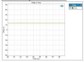
The PESQ: Delay vs Time result is useful for cause analysis. The result shows signal delay time versus elapsed time.
