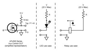
LEDs are typically connected using TTL driver circuits, but can be connected directly as shown above. V and R depend upon the LED selected and other circuit considerations.
