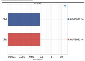
The THD+N Ratio result provides a single-value measurement of the THD+N (total harmonic distortion plus noise) ratio in the output signal from each DUT channel.
