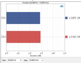
The **Multitone Analyzer: Deviation** result uses the multitone method to provide the frequency deviation (the total range of frequency variation) of each DUT channel, displayed as a meter (single value) result. You can specify a minimum and maximum frequency to define the range to be considered in the deviation measurement.
