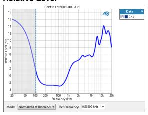
The Relative Level result is a continuous sweep measurement that provides a graphical display of the frequency response of each channel. In this result the DUT output level is plotted against frequency, relative to the level at a selected frequency set in the **Ref Frequency** field.
