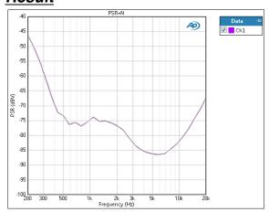
The PSR+N (Power Supply Rejection plus Noise) acquisition is filtered by a weighting filter, if applied. The PSR+N is the RMS level of the broadband result, plotted against frequency.
