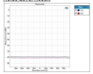
The DC Level Sweep measurement uses a DC stimulus that is moved across a range of values in a series of points. The DUT output is acquired by the analyzer. This view shows the Noise result. The Noise result can be filtered.
