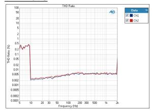
The THD Ratio result uses a fixed audio stimulus signal while the jitter generator is moved across a range of frequencies in a specified number of points. In this result the ratio of the level of the THD (total harmonic distortion) to the total signal in the DUT output is plotted against frequency.
