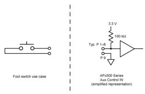
Input switches and sensors are often connected using TTL driver circuits, but can be connected directly as shown above.
