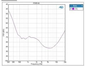
PSRR+N is Power Supply Rejection Ratio plus Noise. This nomenclature is used to describe the ratio of the level of a residual power supply perturbation plus noise found in the output signal, to the AC signal that is the source of perturbation in the power supply. In APx, this result is only available when the analyzer input is analog.
