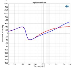
This result provides a graphical display of the impedance phase response of the driver, plotting the impedance phase versus frequency.
