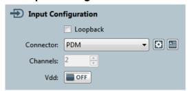
Note: APx measurements are all performed on the baseband audio signal, at the Decimated Rate. However, it is possible to directly view the undecimated PDM bitstream in the Signal Analyzer, when the Signal control is set to PDM Bitstream.
