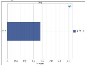
The Acoustic Response Delay result is a single value measurement computed from the impulse response. Delay displays the time delay between the generator output and analyzer input for each channel. For Acoustic Response testing, this is effectively the acoustic delay between the loudspeaker and the measurement microphone.
