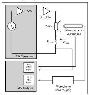
This method uses an external power amplifier and sense resistor. This is the only configuration that supports Loudspeaker Production Test using an analyzer with only two inputs.
