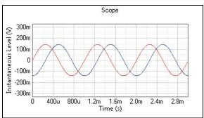
Sine, 1 kHz, 100.0 mVrms. Phase B 90 deg.
