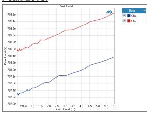
The **Jitter Level Sweep: Peak Level** result uses a fixed audio stimulus signal while the jitter generator is moved across a range of levels in a specified number of points. X axis is generator level; Y axis is the bandpass filtered DUT output level, scaled in peak units.
