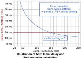
Settling delay calculation.
