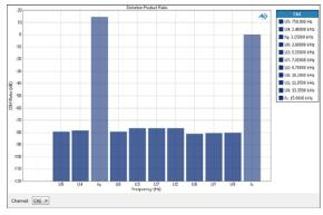
The DIM Distortion Product Ratio result provides measurement results of the IMD (intermodulation distortion) ratio in the output signal from each DUT channel.
