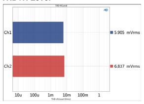
The THD+N Level result provides a single-value measurement of the THD+N (total harmonic distortion plus noise) level in the output signal from each DUT channel.
