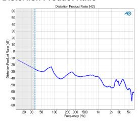
The Loudspeaker Production Test Distortion Product Ratio result is a continuous sweep measurement that provides a graphical display of the selected harmonic distortion products present in each audio input channel. In this result the ratio of the level of the selected harmonic distortion product to the fundamental in the DUT output is plotted against frequency.
