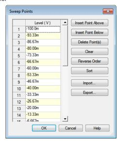
A Linear sweep can include a range that extends into negative values, but a Logarithmic sweep can only include positive values.
