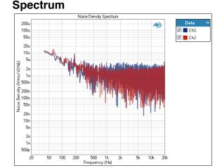
The Multitone Analyzer: Noise Density Spectrum result provides an FFT spectrum display of the acquired signal. All odd-numbered bins that are not within the current Skirt width are plotted in this display; even numbered bins are not reported, ignoring stimulus tones and distortion products. This produces a noise-only result. This result is scaled for display in the accepted unit for noise density results: V/root(Hz) for analog inputs, or FS/root(Hz) for digital inputs.
