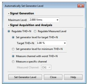
Auto Gen Level uses generator regulation to automatically find the optimum testing level, regulating to your selected Target THD+N or Target Measured Level. Read more about regulation in beginning on page 433.
