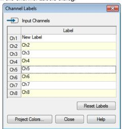
Here you can rename the input channels with names of your choice. These settings are project-wide, but can be overridden for any measurement result.
