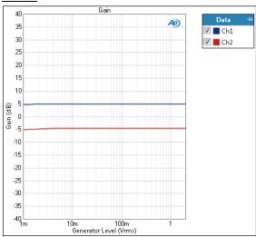
The Bandpass Level Sweep: Gain result uses a sine wave stimulus signal that is moved across a range of levels in a series of points. X axis is generator level; Y axis is gain in the DUT. Gain is a ratio, calculated by dividing the bandpass filtered DUT output level by the generator level.
