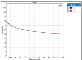
The Jitter Level Sweep: SINAD result uses a fixed audio stimulus signal while the jitter generator is moved across a range of levels in a specified number of points. X axis is generator level; Y axis is DUT output SINAD ratio.
