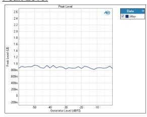
The Stepped Level Sweep: Peak Level result uses a sine wave stimulus signal that is moved across a range of levels in a series of points. X axis is generator level; Y axis is the bandpass filtered DUT output level, scaled in peak units.
