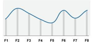
**Multitone: Level** displays a frequency response curve that plots the level across all of the tones at analysis. The amplitudes in the FFT bins that correspond to the multitone stimulus tones are shown as a light gray lines. The dark line represents the frequency response curve.
