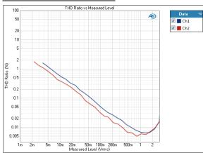
The Stepped Level Sweep: THD Ratio vs. Measured Level result uses a sine wave stimulus signal that is moved across a range of levels in a series of points. X axis is measured DUT output level; Y axis is DUT output THD ratio.
