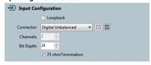
This selection enables the unbalanced digital electrical input, available on a BNC connector on the instrument front panel.
