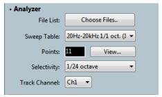
This control is available if the **Input Configuration** in **Signal Path Setup** is set to one of the two **File** choices. Read more about analyzing audio files in Chapter 19.
