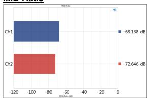
IMD Ratio provides a single-value result showing the IMD (intermodulation distortion) ratio in the output signal from each DUT channel, using the SMPTE, DFD, CCIF or MOD method.
