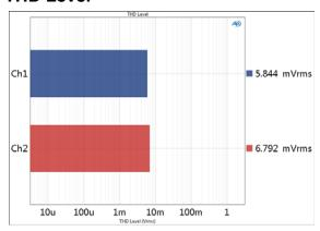
The THD Level result provides a single-value measurement of the THD (total harmonic distortion) level in the output signal from each DUT channel.
