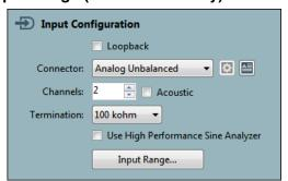
For analog inputs in Bench Mode, the **Input Range...** dialog is available to set input ranging. This feature is available in Sequence Mode in the Advanced Settings dialogs for individual measurements. See Chapter 92, Ranging and Settling.
