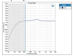
Group delay is a measure of the rate of change of phase shift as a function of frequency. Group delay can also be described as a time delay of a group of frequencies with respect to the generator.
