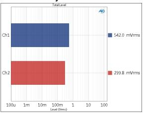
The **Multitone Analyzer: Total Level** result uses the multitone method to provide the total rms level (the sum of the rms levels of all tones and their skirts) for each DUT channel, displayed as a meter (single value) result.
