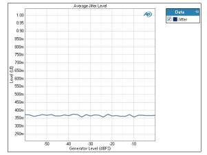
The Stepped Level Sweep: Average Jitter Level result uses a sine wave stimulus signal that is moved across a range of levels in a series of points. X axis is generator level; Y axis is the bandpass filtered DUT output jitter level, scaled in average units.
