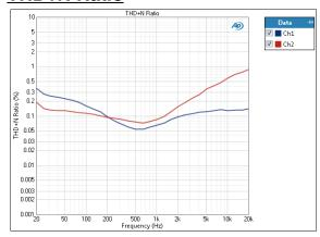
The THD+N Ratio result is a stepped frequency sweep measurement that provides a graphical display of the THD+N response of each channel. In this result the ratio of the level of the THD+N (total harmonic distortion plus noise) to the total signal in the DUT output is plotted against frequency.
