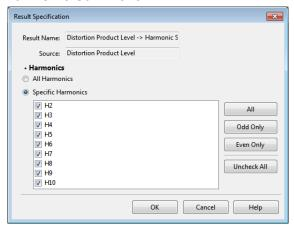
The Harmonic Sum Level derived result can be attached to the THD+N Distortion Product Level result.
