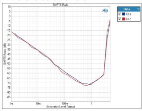
IMD Ratio plots the distortion on the Y axis against the Generator level on the X axis, using the SMPTE, DFD CCIF or MOD IMD method.
