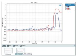
These results show a 10 second recording of Level and THD+N results, while the DUT gain is increased.
