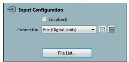
For File Input configuration in Bench Mode, the **File List...** browser is available. This feature is available in Sequence Mode in the Analyzer settings for individual measurements. See Chapter 19, Open Loop measurements.
