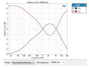
The Multitone Analyzer: Relative Level result uses the multitone method to provide a graphical display of the level vs. frequency (frequency response) for each channel of the DUT, relative to the measured level at a reference frequency. This enables you to specify a frequency that will be set as 0 dB, and to view the response in relation to that frequency. The rms value of each tone is measured, and a response curve is plotted through these values.
