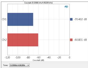
The Multitone Analyzer: Crosstalk (at Tone Pair) result uses the multitone method to provide the crosstalk level for a selected tone pair for each DUT channel, displayed as a meter (single value) result.
