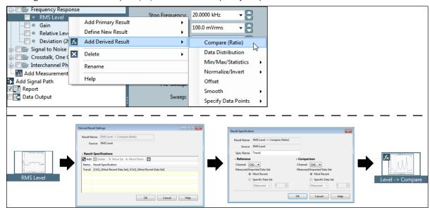
Attaching the Derived Result to the source result opens a Result Settings dialog, where you can specify one or more Result Specifications. We have only one specification, the default, which compares the data in channel 1 with the data in channel 2, for the most recent data set. The Derived Result is of the XY type, with one graph trace for each specification.
