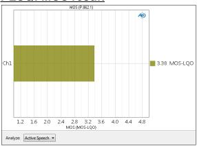
The **PESQ: MOS** result is the primary result for the PESQ measurement. The PESQ score is mapped to MOS-LQO using P.862.1 for narrowband analysis, or P.862.2 for wideband analysis.
