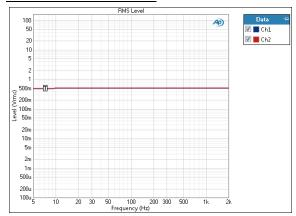
Jitter Frequency Sweep: RMS Level result uses a fixed audio stimulus signal while the jitter generator is moved across a range of frequencies in a specified number of points.
