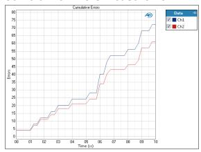
The Digital Error Rate: Cumulative Errors result provides a record of the accumulation of digital errors versus elapsed time.
