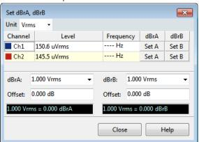
You can save two analog input reference levels and two digital input reference levels for each signal path. These saved input level references are called **dBrA** and **dBrB**, and are independently set for analog and digital inputs. They can be referenced throughout the signal path so that results can be evaluated relative to references. You can set dBrA and dBrB arbitrarily, or you can set them in interaction with your DUT, while observing measured level or distortion.
