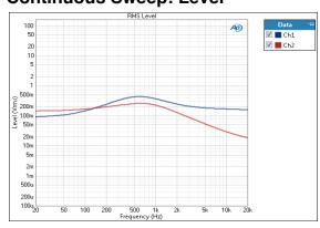
The Level result is a continuous sweep measurement that provides a graphical display of the frequency response of each channel. In this result the DUT output level is plotted against frequency.
