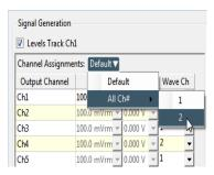
To set individual generator output channel levels, uncheck the **Track first channel** checkbox and enter values in the output channel **Level** fields.
