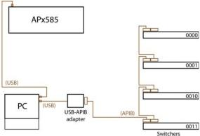
Switcher control interface bus diagram
