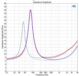
This result provides a graphical display of the impedance response of the driver, plotting the complex impedance magnitude versus frequency. The model fit (Standard model) curve is also plotted on the same graph, shown here as a dashed line.
