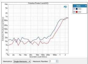
The Stepped Level Sweep Distortion Product Level result provides a graphical display of the selected harmonic distortion products present in each channel. In this result the level of the selected harmonic distortion product in the DUT output is plotted against generator level.
