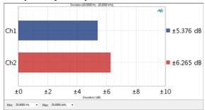
Frequency Response: Deviation is a single value result computed from the continuous sweep acquisition. In this result the frequency deviation (the total range of frequency variation) of each channel is displayed as a meter bar. You can specify a minimum and maximum frequency to define the range to be considered in the deviation measurement.
