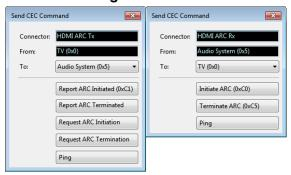
When in an HDMI ARC configuration, the Send CEC dialog allows you to send ARC-related CEC commands to the source or sink device connected.
