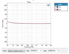
The Continuous Sweep: Phase result displays the DUT output phase for each channel, plotted against frequency. See page 300 for more information about phase measurements.
