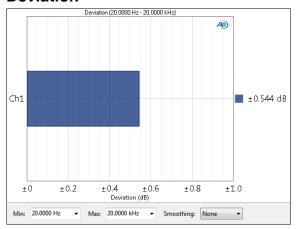
The Acoustic Response Deviation result is a single value measurement computed from the continuous sweep acquisition. In this result the frequency deviation (the total range of frequency variation) of each channel is displayed as a meter bar. You can specify a minimum and maximum frequency to define the range be considered in the deviation measurement.
