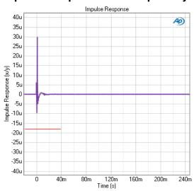
This is a Loudspeaker Production Test Impulse Response result from a system that has correct polarity. The primary impulse is positive. Note the limit set at –18u, to flag reversed polarity.
