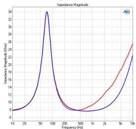
This result provides a graphical display of the impedance response of the driver, plotting the complex impedance magnitude versus frequency.
