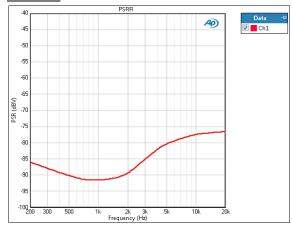
PSRR is Power Supply Rejection Ratio. This nomenclature is used to describe the ratio of the level of a residual power supply perturbation found in the output signal, to the perturbation in the power supply. In APx, this result is only available when the analyzer input is analog.
