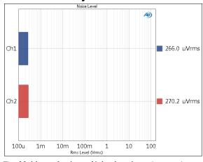
The Multitone Analyzer: Noise Level result uses the multitone method to provide the rms noise level (the sum of the rms noise across the multitone bandwidth) for each DUT channel, displayed as a meter (single value) result. To produce a noise-only result, even-numbered bins and bins in the current Skirt width are excluded from measurement. Instead, such bins are assigned the values in the adjacent odd-numbered bins. All bins are summed.
