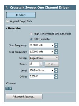
graph data are deleted each time you start a new measurement. If the **Append Graph Data** box is checked, appended data are grouped as additional data sets, as are any imported data. The Data Sets Panel displays the Data Set(s) in the measurement, and provides a visibility checkbox, a Time acquisition field, and a Notes field for each data set.
