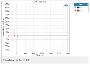
The Impulse Response result is a continuous sweep measurement that displays the impulse response for each channel. Impulse response is plotted against time.
