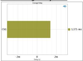
The PESQ: Average Delay result is useful for cause analysis. The result shows the average signal delay through the DUT or system.
