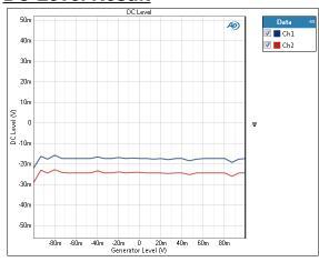
The DC Level Sweep measurement uses a DC stimulus that is moved across a range of values in a series of points. The DUT output is acquired by the analyzer. This view shows DC Level result.
