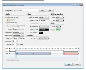
This dialog allows you to set, save or load digital serial transmitter configurations. A dynamic timing diagram provides an on-screen display of your configuration settings. Transmitter connections are provided on an HD-15 connector, with four sets of Master Clock, Bit Clock, Channel Clock and Data connections. A monitor connector provides buffered outputs of these signals for oscilloscope monitoring.
