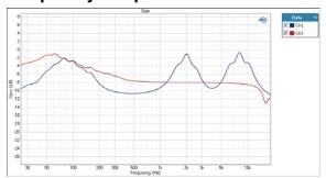
The Frequency Response: Gain result is a continuous sweep measurement that provides a graphical display of the frequency response of each channel. In this result the DUT gain is plotted against frequency.
