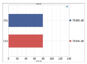
The CMRR Pin 2 and CMRR Pin 3 results are intermediate results, and are provided for diagnostic purposes. Report the data displayed in the CMRR IEC result.
