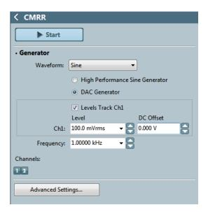
switched to common mode using a pair of matched source resistors, one in each leg of the output circuit. A second measurement is made. The ratio of the two results is displayed as the Common Mode Rejection Ratio (CMRR).
