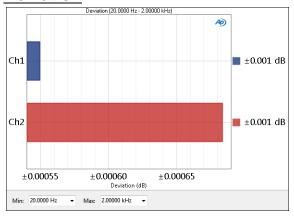
The Jitter Frequency Sweep: Deviation result uses a fixed audio stimulus signal while the jitter generator is moved across a range of frequencies in a specified number of points. This result is a single value mea-
