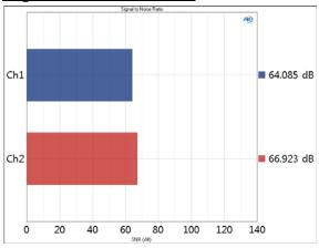
The Signal to Noise Ratio measurement provides a single-value result showing the SNR for each DUT channel.
