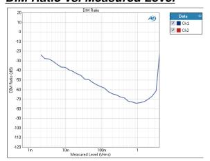
DIM Ratio vs. Measured Level plots the distortion ratio on the Y axis against the DUT output level on the X axis.
