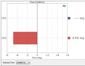
The **Multitone Analyzer: Phase at (Tone)** result uses the multitone method to provide a graphical display of the interchannel phase at any tone in the multitone, for each channel of the DUT. The phase value of the selected tone is measured and compared to the phase value of that tone in the reference channel. Read more about phase on page 300.
