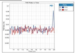
The Measurement Recorder: THD Ratio measurement result provides a record of the THD ratio versus elapsed time for any audio signal. The illustration shows a 20-second record of a 10 kHz sine wave on two channels, with a 10 kHz EQ control adjusted from about -20 dB to about +12 dB during the course of the recording.
