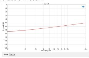
This result shows the crosstalk introduced into Channel 2, while Channel 1 is set as the Source.
