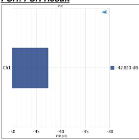
When **AC Waveform** is set to **Sine**, the PSR acquisition is filtered first by a weighting filter, if applied, then by a window width bandpass filter at the sine frequency. The PSR is the RMS level inside the bandpass filter.
