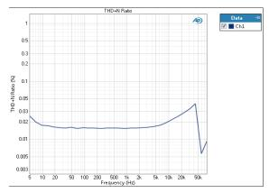
The THD+N Ratio result plots the DUT measured THD+N output Ratio on the Y axis, against the generator frequency on the X axis. This method is often
