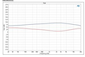
Gain is a Bandpass Frequency Sweep result that provides a graphical display of the voltage gain in each channel. In this result the DUT gain is plotted against frequency. The **Bandpass Frequency Sweep Gain** measurement is not available in **External Source** configuration.
