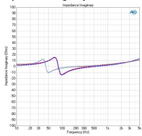
Driver impedance is a complex number, with both real and imaginary components. This result provides a graphical display of the imaginary component of the impedance response of the driver, plotting the imaginary impedance value versus frequency. The dashed line is the model fit trace, here using the Standard model. Traces for **Added Mass** are also shown.
