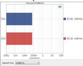
The **Multitone Analyzer: Tone Level** result uses the multitone method to provide the rms level for a selected tone for each DUT channel, displayed as a meter (single value) result.
