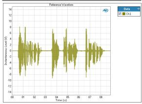
The PESQ: Reference Waveform result is result is useful for cause analysis. The result shows a time-domain view of the reference speech sample waveform.
