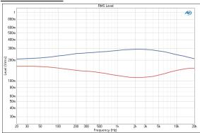
Bandpass Frequency Sweep: RMS Level results uses a sine wave stimulus signal that is moved across a range of frequencies in a specified number of points. This is the conventional frequency response sweep, bandpass filtered.
