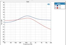
The Gain result is a continuous sweep measurement that provides a graphical display of the frequency response of each channel. In this result the DUT gain is plotted against frequency.
