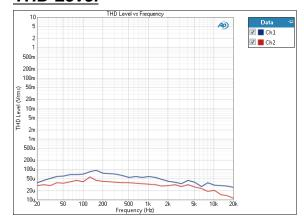
The THD Level result is a stepped frequency sweep measurement that provides a graphical display of the THD response of each channel. In this result the level of the THD (total harmonic distortion) in the DUT output is plotted against frequency.
