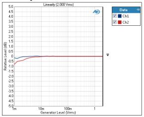
The Bandpass Level Sweep: Linearity result uses a sine wave stimulus signal that is moved across a range of levels in a series of points. X axis is generator level; Y axis is linearity in the DUT. Linearity is a ratio, calculated by dividing the bandpass filtered DUT output level by the generator level, normalized for a chosen relative level.
