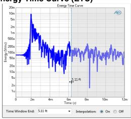
The Energy Time Curve (ETC) provides a graphical display of the ETC of the loudspeaker and acoustic space. This view is useful in setting up an acoustic measurement. See More About the Energy Time Curve on page 185.
