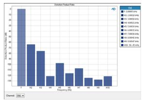
The THD+N Distortion Product Ratio result displays a single-value measurement of the ratio of a distortion product (single harmonic) to the total signal for a selected channel, for the harmonics 2–10. The level displayed in each bar is the rms level of that harmonic tone divided by the rms level of the total signal.
