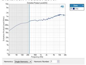
The Acoustic Response Distortion Product Level result is a continuous sweep measurement that provides a graphical display of the selected harmonic distortion products present in each channel. In this result the level of the selected harmonic distortion product in the DUT output is plotted against frequency.
