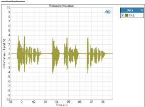
The POLQA: Reference Waveform result is result is useful for cause analysis. The result shows a time-domain view of the reference speech sample waveform.
