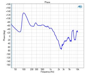
The Loudspeaker Production Test Phase result is a continuous sweep measurement that displays the DUT output phase, plotted against frequency.
