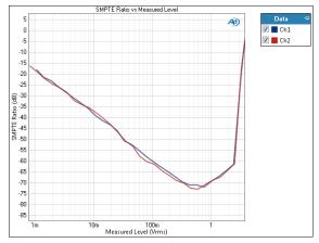
IMD Ratio vs. Measured Level plots the distortion on the Y axis against the measured DUT output level on the X axis, using the SMPTE, DFD CCIF or MOD IMD method.
