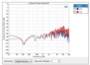
The Continuous Sweep Distortion Product Ratio result is a continuous sweep measurement that provides a graphical display of the selected harmonic distortion products present in each channel. In this result the ratio of the level of the selected harmonic distortion product to the fundamental in the DUT output is plotted against frequency.
