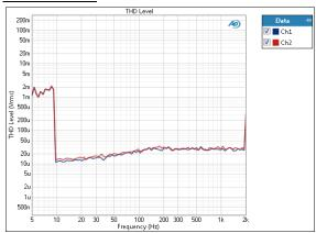
The THD Level result uses a fixed audio stimulus signal while the jitter generator is moved across a range of frequencies in a specified number of points. In this result the level of the THD (total harmonic distortion) in the DUT output is plotted against frequency.
