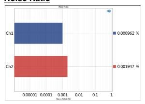
The Noise Ratio result provides a single-value measurement of the Noise ratio in the output signal from each DUT channel.
