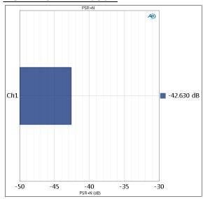
The PSR+N (Power Supply Rejection plus Noise) acquisition is filtered by a weighting filter, if applied. The PSR+N is the RMS level of the broadband result. For the Noise waveform, the PSR and PSR+N results are the same.
