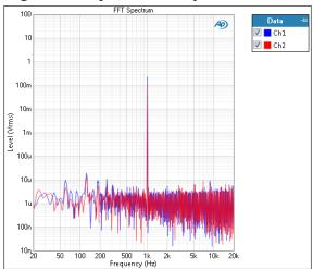
The Signal Analyzer is a general purpose diagnostic tool that uses a high-resolution FFT technique to provide several different display results. FFT Spectrum is a frequency domain result, displaying the signal amplitude versus frequency.
