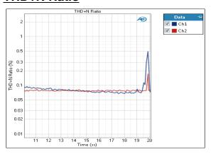
The Measurement Recorder: THD+N Ratio measurement result provides a record of the THD+N ratio versus elapsed time for any audio signal. The illustration shows a 20-second record of a 10 kHz sine wave on two channels, with a 10 kHz EQ control adjusted from about -20 dB to about +12 dB during the course of the recording.
