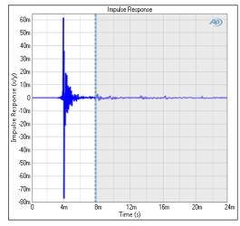
Further confirm by measuring the lengths of the acoustic paths, and obtaining the difference between the direct path and the first reflection path (B+C-A, as shown in the diagram on page 174). That distance should agree closely with the position of the Time Window cursor, when viewed in distance units.
