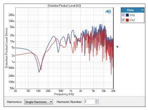
The Continuous Sweep Distortion Product Level result is a continuous sweep measurement that provides a graphical display of the selected harmonic distortion products present in each channel. In this result the level of the selected harmonic distortion product in the DUT output is plotted against frequency.
