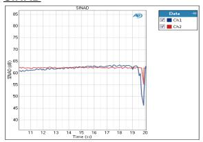
The Measurement Recorder: SINAD measurement result provides a record of the SINAD ratio versus elapsed time for any audio signal. The illustration
