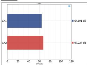
The SINAD measurement provides a single-value result showing the SINAD for each DUT channel.
