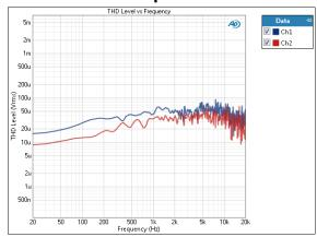
The THD Level result is a continuous sweep measurement that provides a graphical display of the harmonic distortion response of each channel. In this result the level of the THD (total harmonic distortion) in the DUT output is plotted against frequency.
