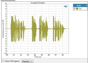
The POLQA: Acquired Waveform result is useful for cause analysis. The result shows a time-domain view of the acquired speech sample waveform.
