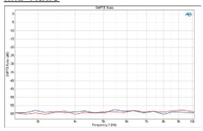
IMD Ratio plots the distortion ratio on the Y axis against the Generator frequency on the X axis, using the SMPTE, DFD, CCIF or MOD IMD method.
