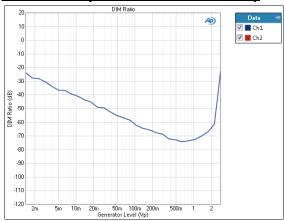
DIM Ratio plots the distortion ratio on the Y axis against the Generator level on the X axis.
