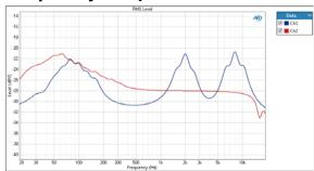
The Frequency Response: Level result is a continuous sweep measurement that provides a graphical display of the frequency response of each channel. In this result the DUT output level is plotted against frequency.
