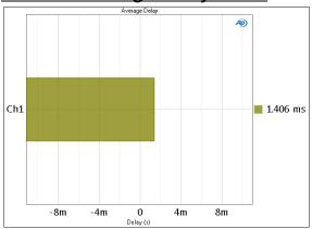
The POLQA: Average Delay result is useful for cause analysis. The result shows the average signal delay through the DUT or system.
