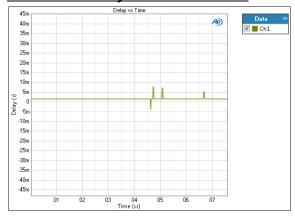
The POLQA: Delay vs Time result is useful for cause analysis. The result shows signal delay time versus elapsed time.
