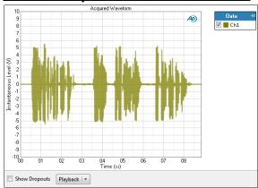
The PESQ: Acquired Waveform result is useful for cause analysis. The result shows a time-domain view of the acquired speech sample waveform.
