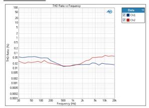
The THD Ratio result is a stepped frequency sweep measurement that provides a graphical display of the THD response of each channel. In this result the ratio of the level of the THD (total harmonic distortion) to the total signal in the DUT output is plotted against frequency.
