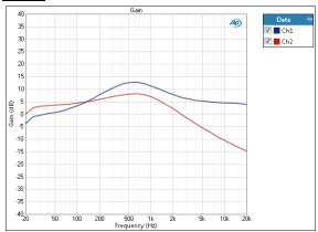
Gain is a stepped frequency sweep result that provides a graphical display of the voltage gain in each channel. In this result the DUT gain is plotted against frequency. The stepped frequency sweep Gain measurement is not available in External Source configuration.
