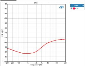
The PSR acquisition is filtered first by a weighting filter, if applied, then by a window-width bandpass filter that is swept at the sine frequency. The PSR is the RMS level inside the bandpass filter, plotted against frequency.
