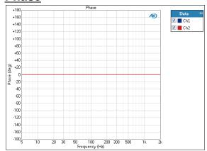
The Phase result uses a fixed audio stimulus signal while the jitter generator is moved across a range of frequencies in a specified number of points. One channel is chosen as the phase reference channel, and the remaining channels are measured against it.
