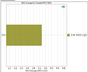
The POLQA: MOS Average result is the primary result for the POLQA (Averaged) measurement. The POLQA score is mapped to MOS-LQO using LC Standard IRS P.863. This result provides an average of all the MOS scores of the speech samples in the Reference Files list.
