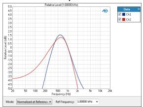
The Relative Level result is a continuous sweep measurement that provides a graphical display of the frequency response of each channel. In this result the DUT output level is plotted against frequency, relative to the level at a selected reference frequency. This enables you to specify the frequency that will be set as 0 dB and view the response in relation to that frequency. A midband frequency such as 1 kHz is often set as the reference frequency, and is the default here.
