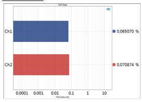
The THD Ratio result provides a single-value measurement of the THD (total harmonic distortion) ratio in the output signal from each DUT channel.
