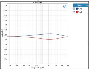
The **Multitone Analyzer: Level** result uses the multitone method to provide a graphical display of the level vs. frequency (frequency response) for each channel of the DUT. The rms value of each tone is measured, and a response curve is plotted through these values.
