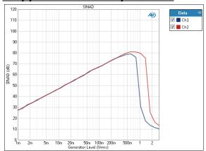
The Stepped Level Sweep: SINAD result uses a sine wave stimulus signal that is moved across a range of
