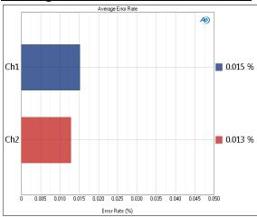
The Digital Error Rate: Average Error Rate measurement result provides a single-value measurement of the average audio bit error rate. The average error rate is calculated by dividing the errors received by the total number of samples received.
