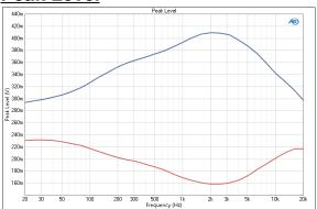
Stepped Frequency Sweep: Peak Level results uses a sine wave stimulus signal that is moved across a range of frequencies in a specified number of points. This is a frequency response sweep, with peak-scaled results.
