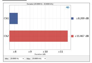
The Stepped Frequency Sweep: Deviation result uses a sine wave stimulus signal that is moved across a range of frequencies in a specified number of points. This result is a single value measurement computed from the stepped sweep that shows the frequency deviation (the total range of frequency variation) of each channel as a meter bar. You can specify a minimum and maximum frequency to define the range of the deviation measurement.
