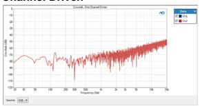
The Crosstalk, One Channel Driven result provides a graphical display of the crosstalk from a selected source channel into each of the other channels. See page 238 for more information about crosstalk.
