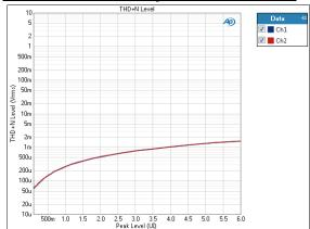
The Jitter Level Sweep: THD+N Level result uses a fixed audio stimulus signal while the jitter generator is moved across a range of levels in a specified number of points. X axis is generator level; Y axis is DUT output THD+N level.
