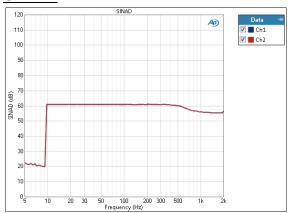
The Stepped Level Sweep: SINAD result uses a fixed audio stimulus signal while the jitter generator is moved across a range of frequencies in a specified number of points. X axis is generator level; Y axis is DUT output SINAD ratio.
