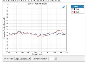
The Stepped Frequency Sweep Distortion Product Ratio result provides a graphical display of the selected harmonic distortion products present in each channel. In this result the ratio of the level of the selected harmonic distortion product to the fundamental in the DUT output is plotted against frequency.
