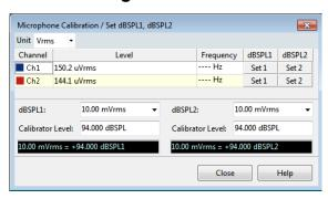
Typically, dBSPL is referenced to a measurement microphone and a microphone calibrator, in APx External Source configuration, without using the APx generator
