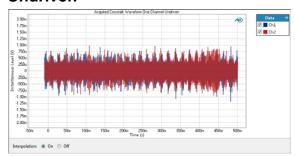
The Acquired Crosstalk Waveform, One Channel Undriven result is a continuous sweep measurement that displays the Acquired Crosstalk Waveform for each channel. This acquisition is only made when Crosstalk Mode is set to **High Accuracy, One Channel Undriven**. See page 220 for more information about acquired waveform.
