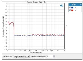
The Jitter Frequency Sweep Distortion Product Ratio result uses a fixed audio stimulus signal while the jitter generator is moved across a range of frequencies
