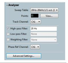
The analyzer Sweep Table menu, and the Points, View/Edit and Track Channel controls discussed below, are not shown for a closed loop sweep that uses the internal generator. In that case, the stimulus sweep definition is directly available to the analyzer and these controls are unnecessary.
