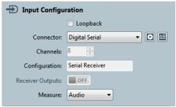
This Connector selection enables the Digital Serial input available on the Receiver HD-15 connector on the instrument front panel; also, the parallel buffered receiver Monitor output is enabled.
