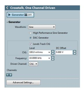
The generator outputs the test signal on one channel only, called the "Driven Channel." The crosstalk (signal leakage) in each of the remaining channels is measured.
