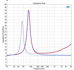
Driver impedance is a complex number, with both real and imaginary components. This result provides a graphical display of the real component of the impedance response of the driver, plotting the real impedance value versus frequency. The dashed line is the model fit trace, here using the Standard model. Traces for **Added Mass** are also shown.
