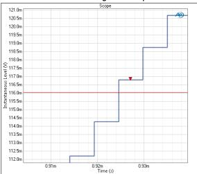
Limit failure marker on data with interpolation ON.
