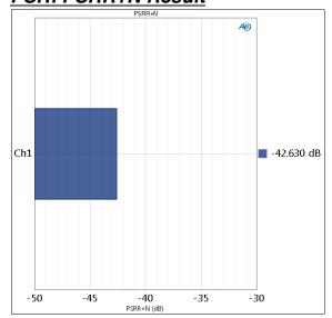
PSRR is Power Supply Rejection Ratio plus Noise. This nomenclature is used to describe the ratio of the level of a residual power supply perturbation plus noise found in the output signal, to the AC signal that is the
