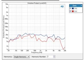
The Stepped Frequency Sweep Distortion Product Level result provides a graphical display of the selected harmonic distortion products present in each channel. In this result the level of the selected harmonic distortion product in the DUT output is plotted against frequency.
