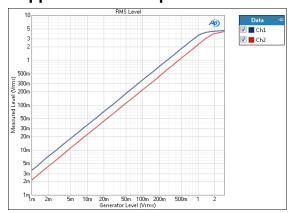
The Stepped Level Sweep: Level result uses a sine wave stimulus signal that is moved across a range of levels in a series of points. X axis is generator level; Y axis is DUT output level.
