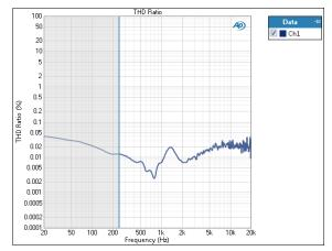
The THD Ratio result is a continuous sweep measurement that provides a graphical display of the harmonic distortion response of each channel. In this result the ratio of the level of the THD (total harmonic distortion) to the total signal in the DUT output is plotted against frequency.
