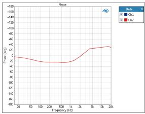
The **Multitone Analyzer: Phase** result uses the multitone method to provide a graphical display of the interchannel phase vs. frequency (interchannel phase response) for each channel of the DUT. The phase value of each tone is measured and compared to the phase value of the reference channel at the same tone, and a response curve is plotted through these values.
