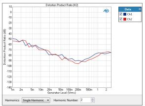
The Stepped Level Sweep Distortion Product Ratio result provides a graphical display of the selected harmonic distortion products present in each channel. In this result the ratio of the level of the selected harmonic distortion product to the fundamental in the DUT output is plotted against generator level.
