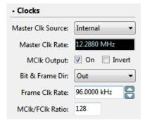
Transmitter Settings: Master Clk Internal, Bit & Frame Out
