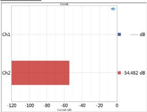
The Crosstalk measurement result provides a single-value measurement crosstalk in the DUT. In this case, the Driven Channel is Channel 1, so crosstalk results only appear in Channel 2.
