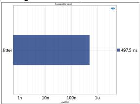
Average Jitter Level provides a single-value meter result, displaying the average jitter level from the digital receiver.
