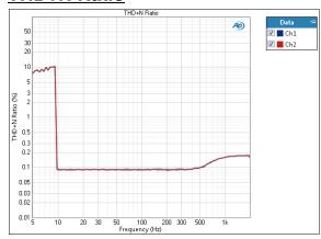
The THD+N Ratio result uses a fixed audio stimulus signal while the jitter generator is moved across a range of frequencies in a specified number of points. In this result the ratio of the level of the THD+N (total harmonic distortion plus noise) to the total signal in the DUT output is plotted against frequency.
