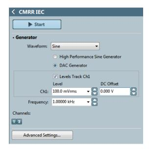
cally switched to use an IEC-defined common mode circuit, where one leg of the output circuit is connected directly to the generator output and the other leg is connected through an additional 10 ohm source resistor. A second measurement is made. Then the resistor and the direct connection are exchanged, and a third measurement is made. The worst ratio is reported as the CMRR IEC measurement result.
