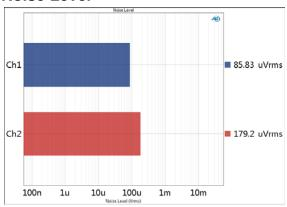
The Noise Level result provides a single-value measurement of the Noise level in the output signal from each DUT channel.
