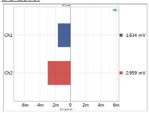
The DC Level measurement provides a single-value result showing the DC voltage present at the output of each DUT channel.
