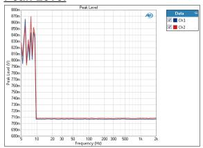
Jitter Frequency Sweep: Peak Level result uses a fixed audio stimulus signal while the jitter generator is moved across a range of frequencies in a specified number of points. This is a frequency response sweep, with peak-scaled results.
