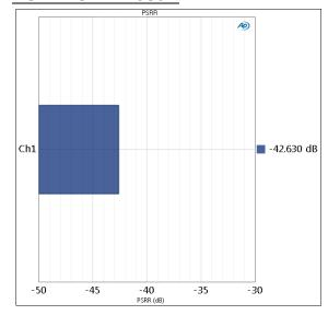
PSRR is Power Supply Rejection Ratio. This nomenclature is used to describe the ratio of the level of a residual power supply perturbation found in the output signal, to the perturbation in the power supply. In APx, this result is only available when the analyzer input is analog.
