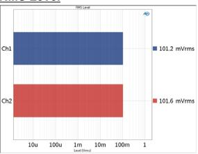
RMS Level provides a single-value meter result, displaying of the rms output level from each DUT channel, as measured at each analyzer input.
