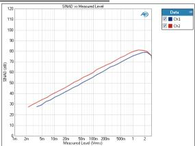
The Stepped Level Sweep: SINAD vs. Measured Level result uses a sine wave stimulus signal that is moved across a range of levels in a series of points. X axis is measured level; Y axis is DUT output SINAD ratio.
