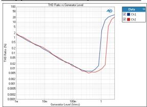
The Stepped Level Sweep: THD Ratio result uses a sine wave stimulus signal that is moved across a range of levels in a series of points. X axis is generator level; Y axis is DUT output THD ratio.
