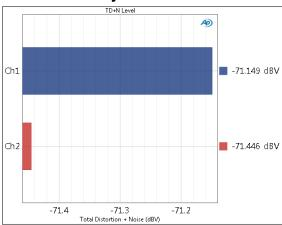
The **Multitone Analyzer: TD+N Level** result uses the multitone method to provide the rms total distortion + noise level (the sum of the rms distortion + noise across the multitone bandwidth) for each DUT channel, displayed as a meter (single value) result. To produce a total distortion + noise result, tone bins and bins in the current **Skirt width** are excluded from measurement. All other bins, odd and even, are summed.
