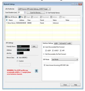
This dialog provides settings for Bluetooth discovery, pairing, connection and other configuration. Unlike most APx settings, Bluetooth profile selection, pairing and connection settings are global to the APx project. Settings made here affect both Bluetooth source and sink configurations across all signal paths in the project.
