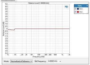
The Jitter Frequency Sweep: Relative Level result uses a fixed audio stimulus signal while the jitter generator is moved across a range of frequencies in a specified number of points. Additionally, in this result the
