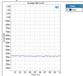
The Measurement Recorder: Average Jitter Level result uses a sine wave stimulus signal that is moved across a range of levels in a series of points. X axis is generator level; Y axis is the bandpass filtered DUT output jitter level, scaled in average units.
