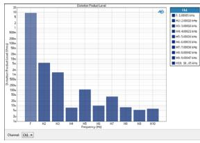
The THD+N Distortion Product Level result displays a single-value measurement of the rms level of distortion products (harmonics) for the harmonics 2–10. The level displayed in each bar is the rms level of that harmonic tone.
