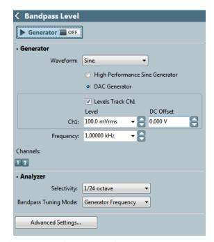
See Chapter 5 for detailed information about the using the APx Generator and making Waveform, Level and Frequency settings, or for information about using External Source.
