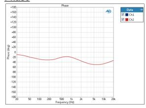
The Phase result is a stepped frequency sweep measurement that provides a graphical display of the Phase response of each channel. One channel is chosen as the phase reference channel, and the remaining channels are measured against it.
