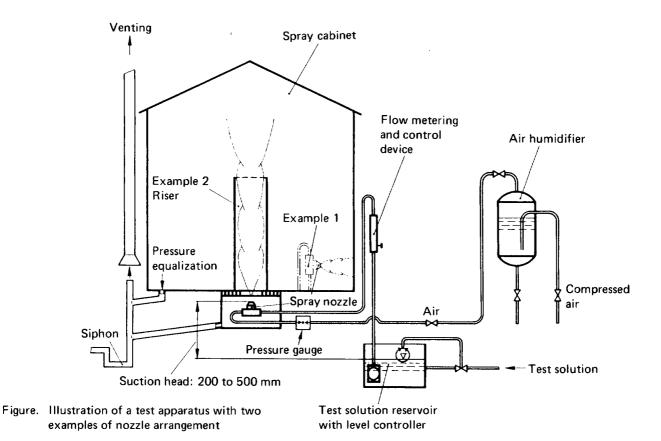
The useful space for test purposes is limited to that part of the cabinet which lies outside the spray jet and in which a uniform dispersion of the spray can be verified as described in subclause 7.2, third paragraph.
