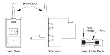
Note: A non-operator-replaceable fuse exists inside of the equipment. This fuse is rated T 40mA 250V,  $5 \times 20mm$ .
