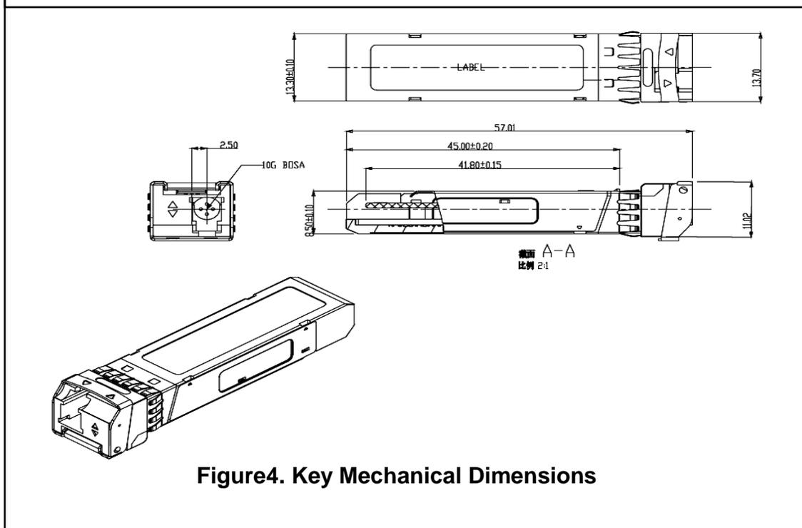
Figure4. Key Mechanical Dimensions
