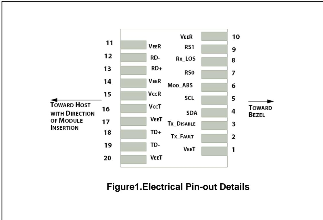
Figure1.Electrical Pin-out Details
