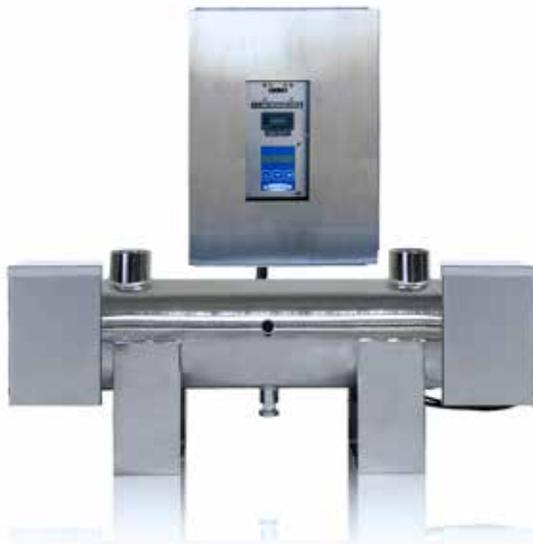
**MODEL SHOWN:** Optima HX Mini 02 BDM U // **INDUSTRIES:** Food & Beverage, Life Sciences, Microelectronics // **FLOWRATES:** 9-33GPM @ 94%UVT, 10-39GPM @ 99%UVT // **APPLICATIONS:** Disinfection, Ozone Destruction // **DESIGN CAPABILITIES:** Custom Configurations
