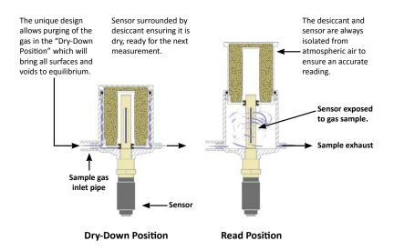
Keeping the sensor dry between tests ensures that the SDHmini-Ex is ready to carry out rapid spot checks. The unique design of the desiccant head achieves this by surrounding the sensor with desiccant, keeping the sensor dry. The head is then lifted for sampling, exposing the sensor to the sample gas.
