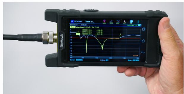
Clearly confirm whether antenna and/or cable lines require replacement with on-screen indicators.
