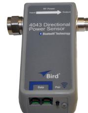
Sensors on both the input and output side of the **COMBINER** enable combiner performance to be measured continuously.
