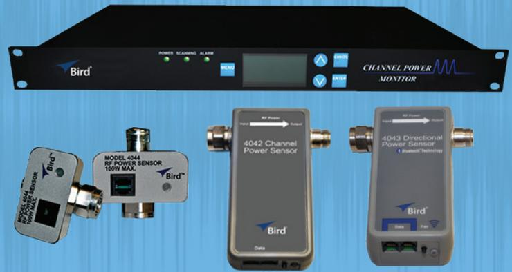
Be assured that your communication system is up and running at all times with Bird's new Channel Power Monitor. It provides you with continuous information on the health of each component of your system that is accessible on any computer or tablet on the network or even the phone in your pocket.
