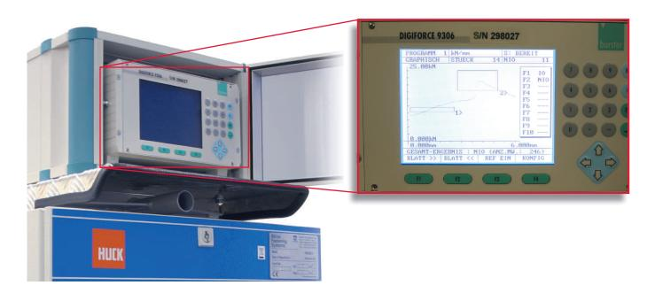
The windows shown on the graphs below are based on data input by the user. The user can specify the entry and exit point for each window. If the curve enters and leaves each window through the specified points then the installation has been successful and the line is drawn in green (graph A).
