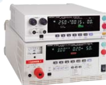
Model 3157-01 AC GROUNDING HiTESTER
