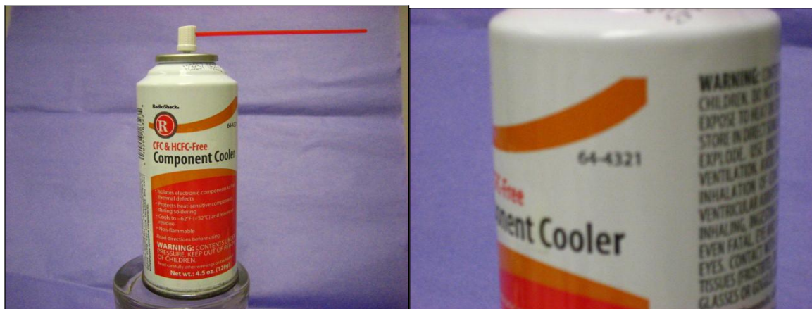
Figure 9 a, b -- Commercial component cooler spray freezes moisture out of the ambient air, simulates detectable ice.
