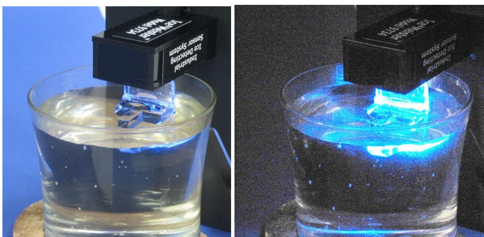
Figure 7 a, b-- CLEAR ICE test with 9-volt battery and clear glass tumbler of clean tap water.
