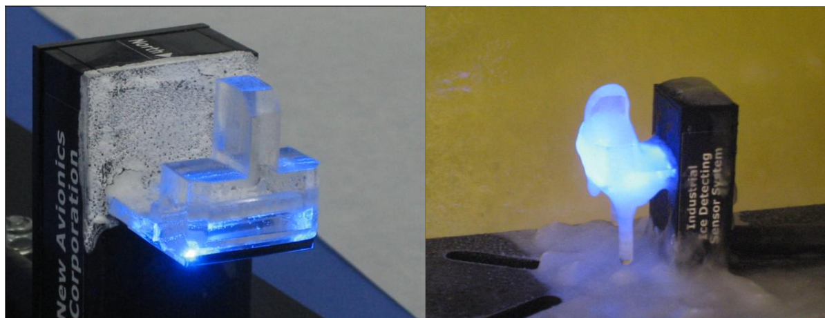
Figure 2 a, b -- Ice*Meister™ Model 9734-SYSTEM senses rime ice, frost etc (left) and clear ice (right).
