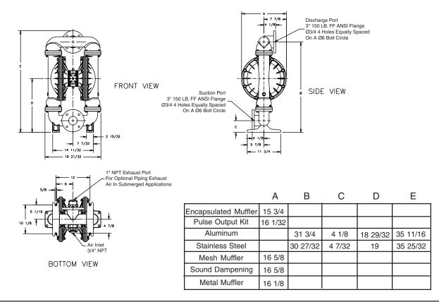
Dimensions in Millimeters Dimensional Tolerance: ±3mm
