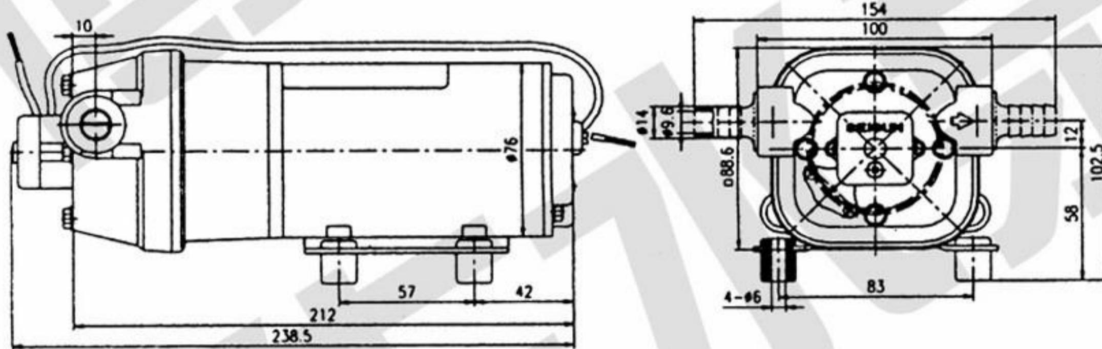
DP-35 (铁底座、橡胶脚柱)
