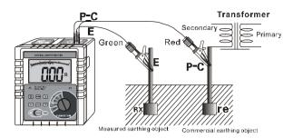
Simple method for measurement of earth ground resistance, its reading on Tester is the total value of earth ground resistance value of measured earthing object and that of commercial earthing object, namely:
