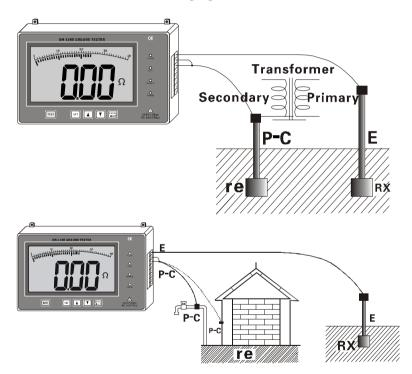
Simple method for measurement of ground resistance, its reading on detector is the total value of ground resistance value of measured grounding object and that of commercial grounding object, namely: In which: RE is the Tester reading value;
