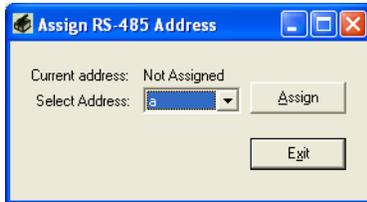
The Connections Menu includes an option that allows you to assign an address to a unit. When you select the Assign ULS Address option, a window will open showing the address that is currently assigned to the connected unit. If no value is assigned or if you want to change the value of the address, use the drop-down menu to display and select the address you want to assign to the unit. The selected address will only be assigned, once you press the Assign button.
