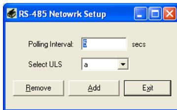
The Connections Menu also includes an option that allows you to modify the RS485 network. This option is used to tell the ULS Interface Program what ULS units are in the network. This option also allows you to add or remove units from the network.
