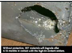
Without protection, SST materials will degrade after 6-18 months in contact with the high-tin content solders.
