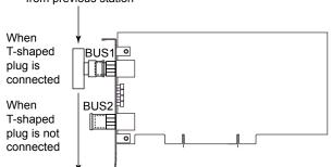
Connect control bus cable to next station (Connect a terminator when next station is not used)
