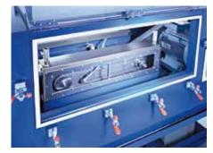
Testing of chain wear elongation behaviour on more than 20 testig rigs
