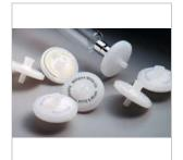
This 25 mm syringe filter with a Hydrophobic PTFE membrane, for non-sterile filtration, has a 0.45 µm pore size used in clarification of organic solvents. Comes in a pack of 250.
