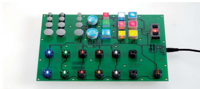
Top half: RAFI short-travel keyswitches RACON 8/12, MICON 5, RF 15/19, short-travel mains switch KN 19 Bottom half: RAFIX FS contact blocks, some with 3 mm THT LEDs
