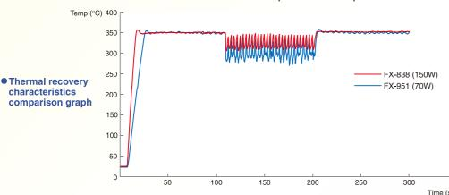
[ Test criteria ] ● Tip shape: 2.4D Board: Paper phenol copper Solder: ø1.6 x 5mm Cycle: Every 3 sec. ● Lead-free solder is used.
