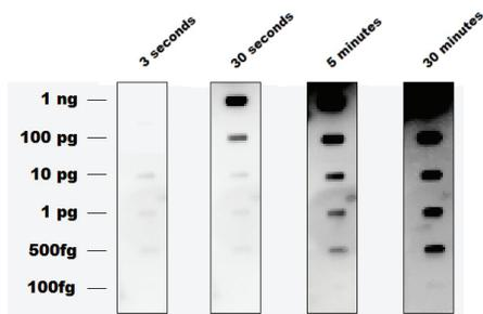
Figure 2: Dilution series showing effect of extending exposure times to 30 minutes on a chemiluminescent slot blot imaged with the FluorChem HD2 system. The capability to detect small quantities of protein (500 fg) increases with increased exposure time when using digital imaging.
