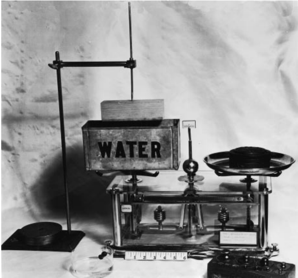
FIG. 39 Specific Gravity and Shrinkage-in-Volume Test Set-Up
