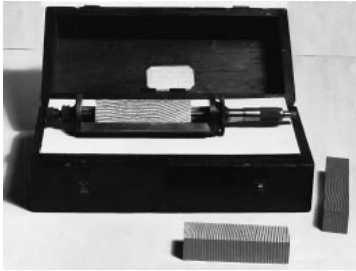
FIG. 41 Radial- and Tangential-Shrinkage Test Assembly
