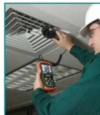
AN100 and AN200 used in HVAC applications measuring airflow from heating vents.
