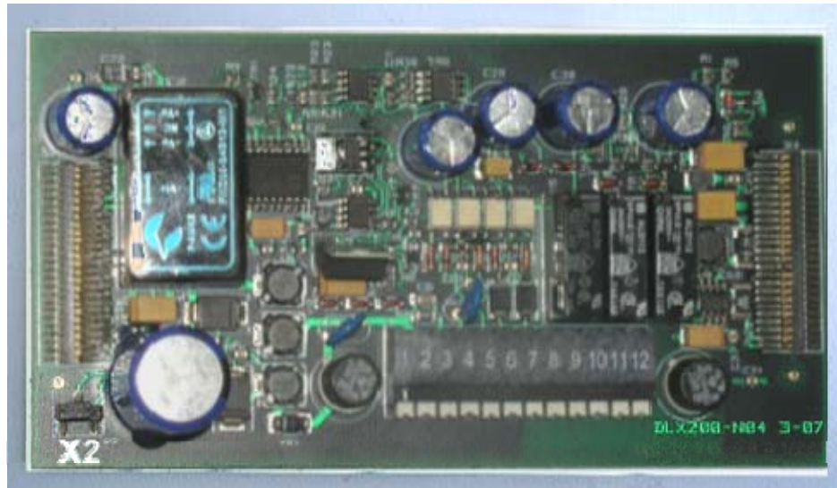
Figure 8.1: PCB no.4, jumper X2"
