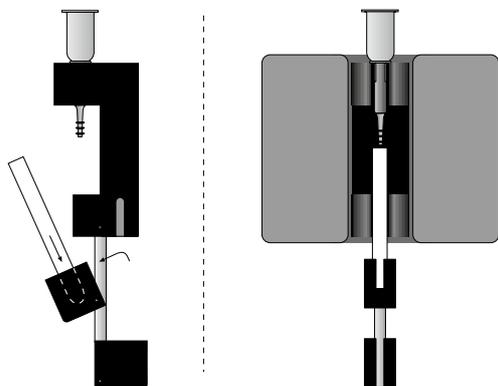
Insert Adapter for MS, LS, and LD Columns in the magnetic field of the SuperMACS™ II Separator (for details, see SuperMACS II data sheets). Place the Column Adapter and the 5 mL collection tube in the upper tube holder.
