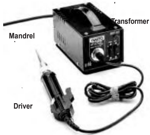
Transformer plugs into standard 110VAC outlet.
