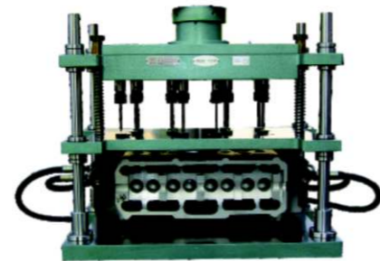
缸体加工,侧面定位,双油缸夹紧 Cylinder process, side locate and doublecylinder clamp
