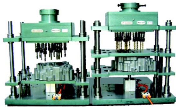
一钻一攻双头机,配合夹具,加工气缸盖 Double head machine with one drill and one tap can process cylinder head using a jig.
