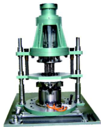
U型固定式,配合油压卡盘 (工件硬度28-32HRC) U-type fixed model, with oil pressure chuck (workpiece rigidity: 28-32HRC)
