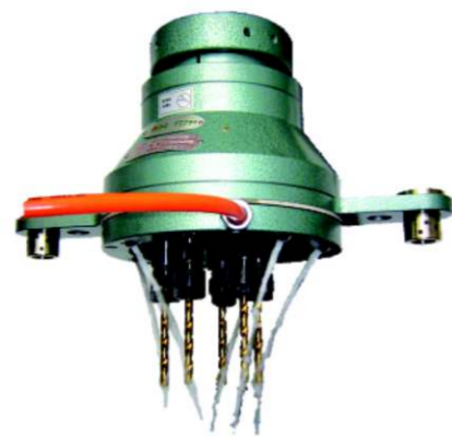
冷却系统与多轴器的结合 Combination of cooling system and multi-spindle head
