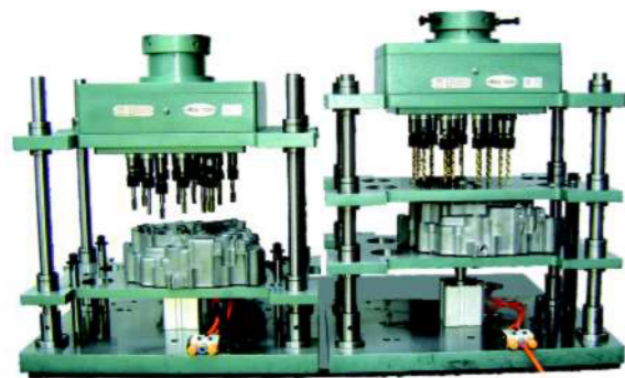
一鑽一攻雙頭機,配合治具,加工氣缸蓋 Double head machine with one drill and one tap can process cylinder head using a jig.
