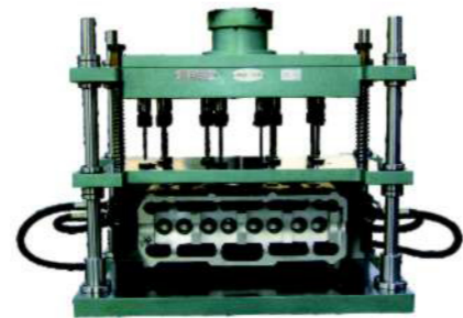
缸體加工,側面定位,雙油缸夾緊 Cylinder process, side locate and double cylinder clamp
