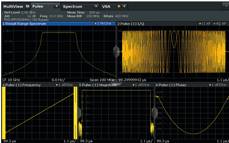
Chirped signal with a duration of 10 µs and a bandwidth of 30 MHz generated with the multifunction generator (R&S®SMAB-K24 option) in the R&S®SMA100B.
