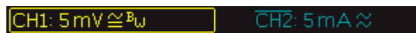
Figure 4-1: Channel labels: Channel 1 is selected, is DC coupled and bandwidth limited. Channel 2 is AC couples and inverted.
