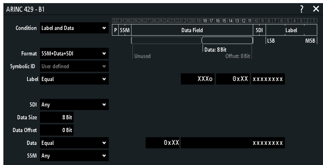
Figure 12-49: Settings for search on ARINC 429 bus
