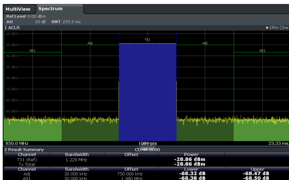
Figure 6-21: Measuring the channel power and adjacent channel power ratio for CDMA2000 signals with zero span (Fast ACLR)
