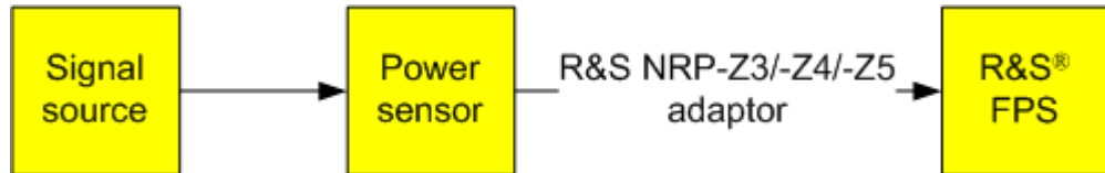
Figure 7-1: Power sensor support – standard test setup
