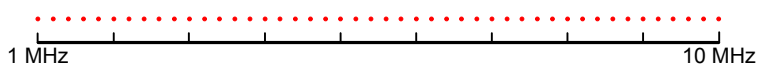
Figure 7-13: Linear x-axis scaling: the distance between the sweep points is equal, e.g. 200 kHz
