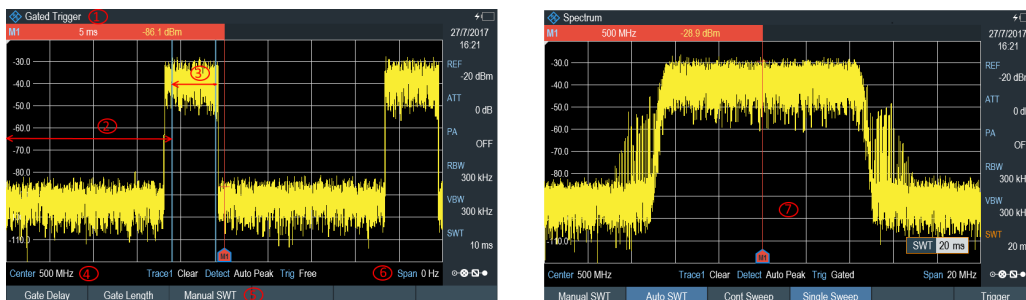
Figure 6-11: Gate trigger measurement
