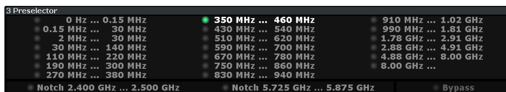
Figure 8-5: Preselector result display. The green LED indicates the currently applied filter.
