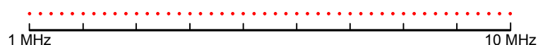
Figure 8-6: Linear x-axis scaling: the distance between the measurement points is equal, e.g. 200 kHz
